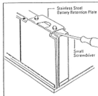
**Step 2.** With the battery removed, adjust both sides of the battery retention plate. Using pliers, slightly raise the bent edges. Adjust the bent edges of the plate so the battery remains secure but can easily be removed.
