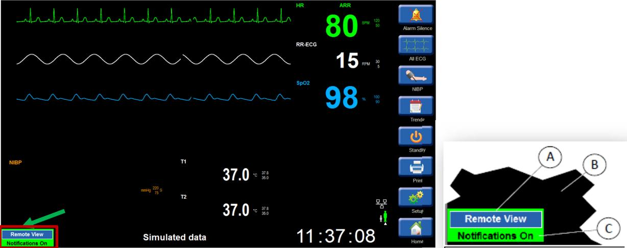
FIGURE 93. Remote View Indicator on Surveyor S12/S19 Home Screen
