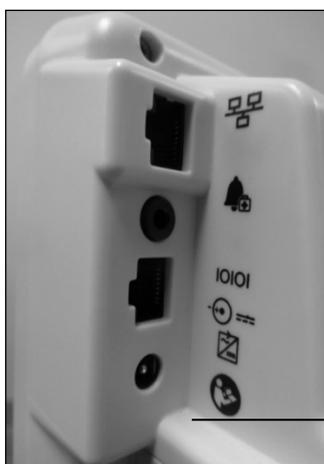
The top corner of the back of the Surveyor S12 and S19 contains the communication ports, an opening for the audio speaker as well as a connection for CO<sub>2</sub> exhaust.
