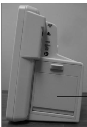
The right side of the Surveyor S12 may contain the optional integrated dual channel thermal recorder (1).
