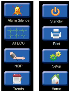
The quick-action keys provide rapid access to commonly used functions.
