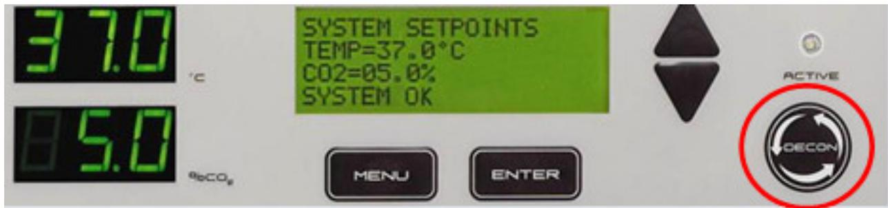
When you are then prompted to remove the IR CO<sub>2</sub> and O<sub>2</sub> sensor (model 6404) press ENTER button to advance to next prompt on screen.
