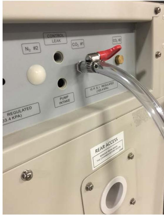
If the unit is equipped with an optional built in gas guard system, there will be 2 gas inlets. Each of the inlets should be connected to an individual gas tank as described above.
