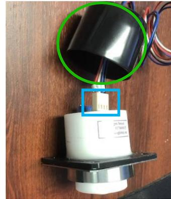
Disconnect the wiring by gently pulling the wiring harness from the small plastic rectangular, flat piece (item in blue square above). Black cover and wiring harness will get tucked back inside of incubator and can stay there during the decon cycle.
