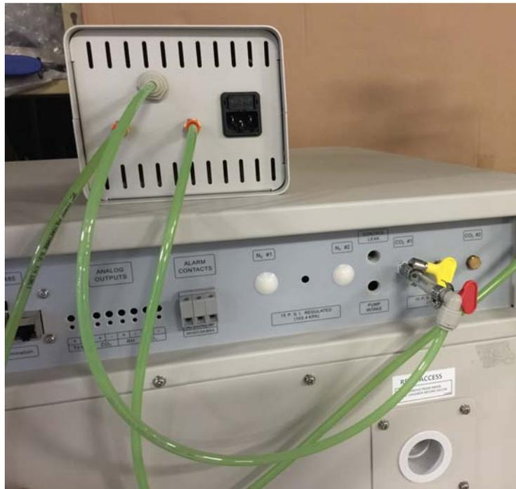
Next, connect the tubing from the outlet of the Gas Guard to the inlet on the back of the chamber as shown in the previous picture. If one or more Gas Guards are supplying separate chambers, the line configuration should be assembled as shown for in the picture below.
