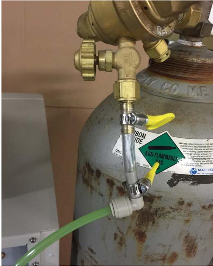
Once the provided tubing is attached to the cylinder regulators, insert the tubing into both Tank 1 and Tank 2 inlets.
