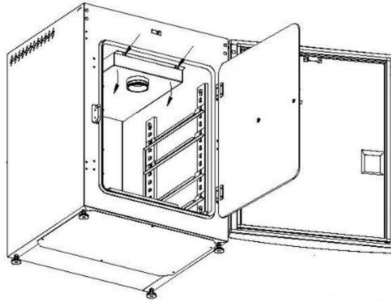
Remove IR CO<sub>2</sub> sensor assembly, grab the silver, knurled holder attached to the grey sensor and pull from retainer clip. Do not touch sensor tip area.
