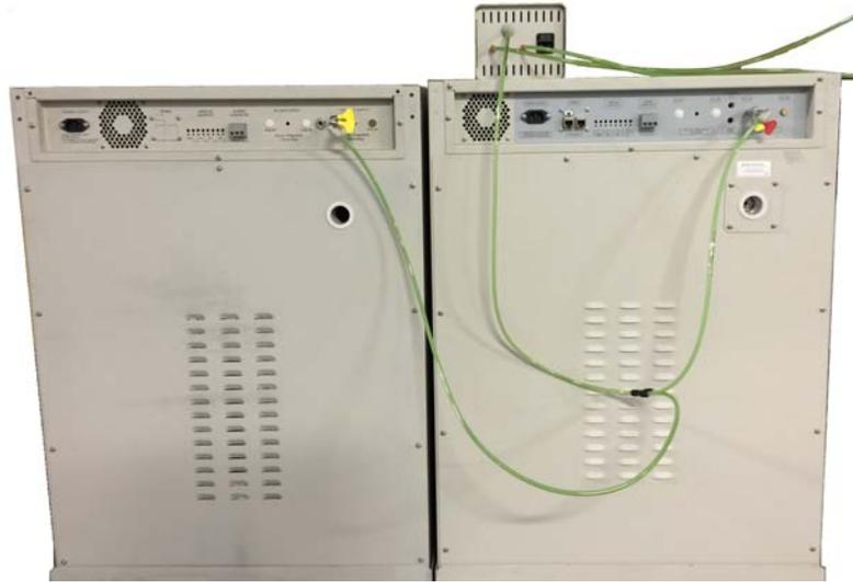
The gas guard is designed to automatically switch from the primary tank to the secondary tank when low gas pressure is detected on the primary tank. This allows for a temporary uninterrupted supply of CO<sub>2</sub> or N<sub>2</sub> to the incubator should the primary tank go empty.
