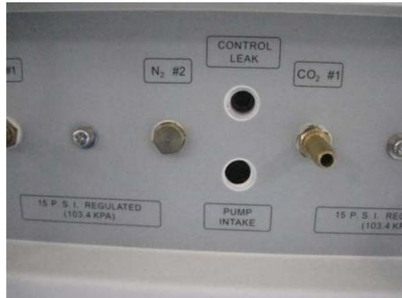
If higher humidity levels higher than 90% are required, install the brass plug that is supplied in the accessory kit into the rear panel of the cabinet labeled Control Leak. This will disable the filtered air exchange. With the filtered air exchange disabled, the humidity level may increase above saturation resulting in some condensation developing on incubator surfaces.
