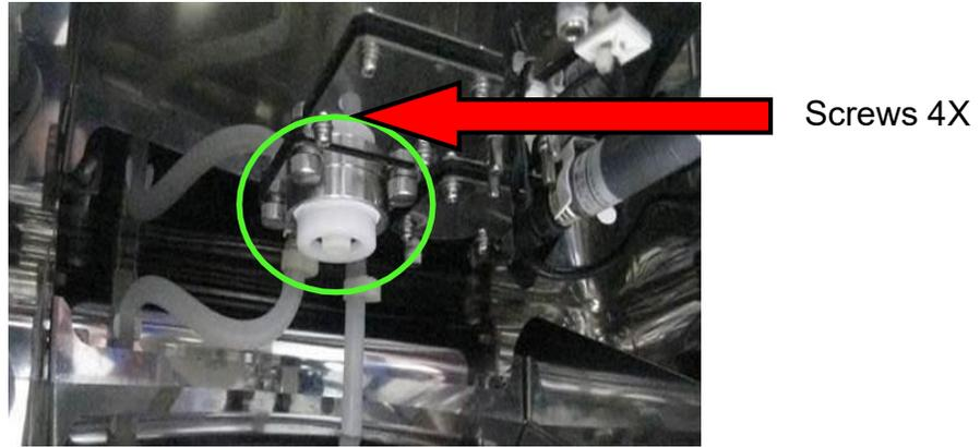
Pull out O<sub>2</sub> sensor gently (sensor as it appears when pulled from inside of incubator is circled in yellow below), as it is attached with a wiring harness internally. Then pull back black cover from O<sub>2</sub> sensor (cover is item circled in green below.).
