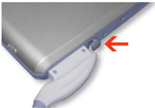
Figure 1-9: Probe Connection Locking Lever
