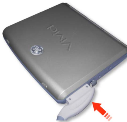
Figure 1-8: Probe Connection to the Vivid i
