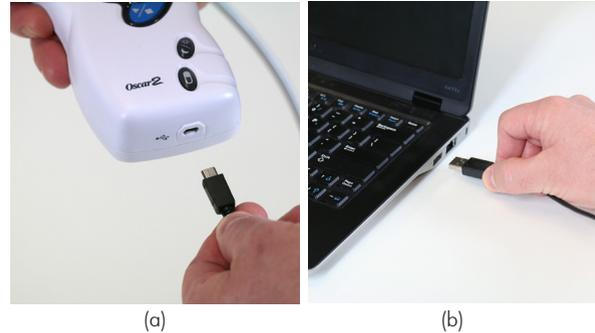
Figure 1: Connecting the Oscar 2 to a PC
