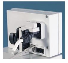
Thanks to the integrated ventilation valve the evaporation can be stopped at any time at the press of a button. The valve is open when not powered so that overpressure in the system is prevented. Only PEEK and Kalrez® materials are used to ensure the highest possible chemical resistance.
