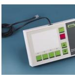
The remote control can be used to operate the vacuum controller and the Rotavapor: rotation, starting/stopping and raising and lowering of the flask.
