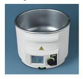
Oval bath pan, incl. base with power supply. Also suitable for use as stand-alone heating bath for thermostatting.
