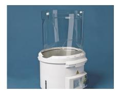
The transparent safety guard is ideally matched to the design of the heating bath and is easy to fit. This accessory provides effective protection for the user against splashing or a possible flask breakage.
