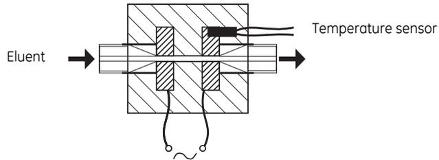
One of the electrodes has a small temperature sensor for measuring the temperature of the eluent in the flow cell. Temperature variations influence the conductivity and in some applications, when highly precise conductivity values are required, it is possible to program a temperature compensation factor that recalculates the conductivity to a set reference temperature.
