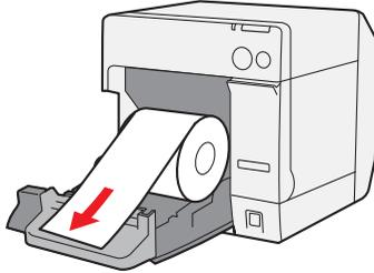
3. While aligning the roll paper with the paper ejection guide, close the roll paper cover.
