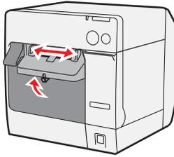
When you install fanfold paper for the first time, or when the paper width needs to be changed, continue to steps 3 and 4.
