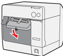
2. Slide the paper ejection guide as wide as possible, and lock it.
