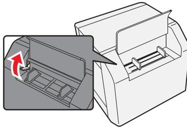
4. Slide the fanfold paper guide to align it with the fanfold paper width, and lock it.
