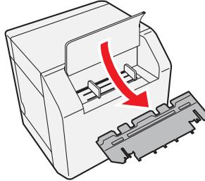
2. Pull the release lever to open the roll paper cover.
