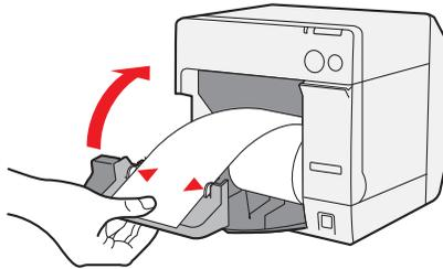
4. Turn on the printer, and then the paper is fed automatically.
