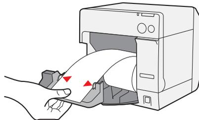
7. Lock the paper ejection guide, and then close the roll paper cover.
