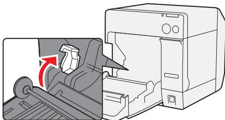
3. Push the roll paper guide on the left in the direction of the arrow, and load the roll paper with the printable side up completely inside the printer.
