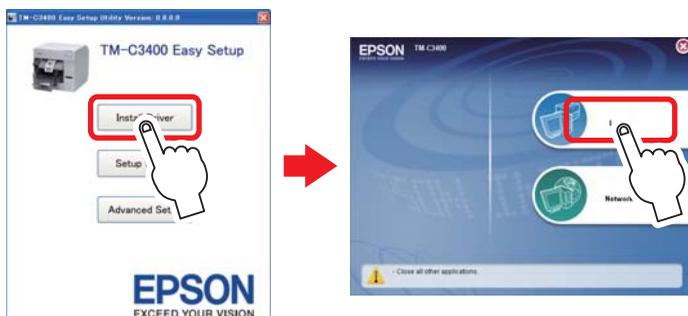
4. Complete the installation by following the instructions displayed. If the screen confirming the connection to the computer is displayed during the installation, turn on the printer.
