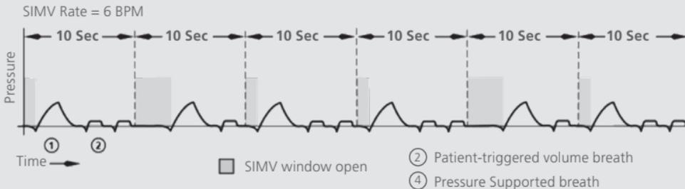
The breath interval is established by the preset breath rate. It resets as soon the interval time has elapsed, or when the **Manual Breath** button is pressed.
