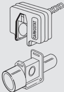
The airway adapter is placed inline between the patient wye and elbow.
