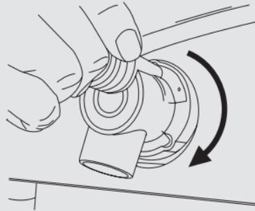
4. Attach the flow sensor with the flow tubes in an upright position.
