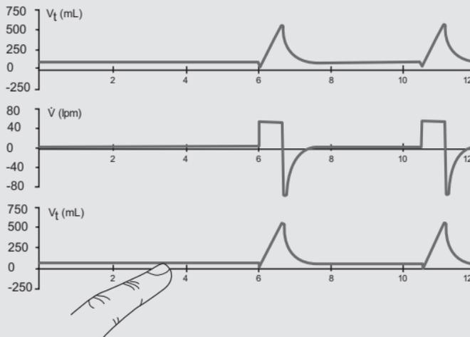
2. Turn the data dial to adjust scale or sweep speed. Touch the axis again, or press the **Accept** button to confirm the changes.
