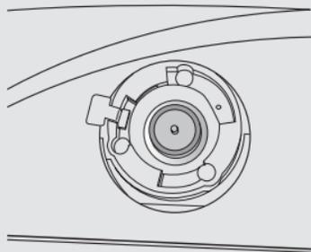
2. Line up the fins of the exhalation valve body with the openings in the exhalation valve housing.
