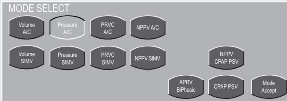
The choices displayed in the Mode Select screen are a combination of breath type and ventilation delivery mode.
