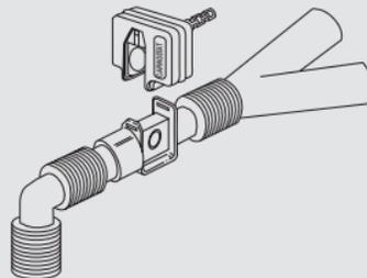
The Capnostat sensor snaps in directly over the airway adapter.
