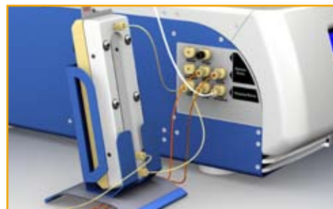
One of Wyatt's AF4 separation channels connected to the Eclipse controller chassis.
