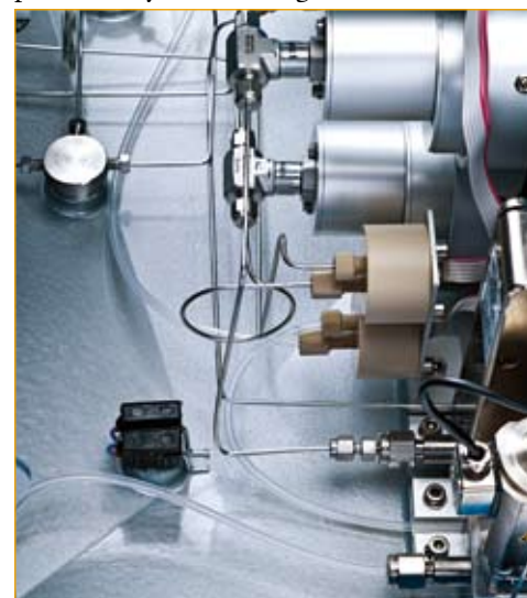
Detailed view of the pressure sensors, leak sensor, and drain pan shown for the organic version with SS tubing.
