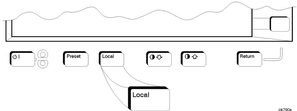
Press this key to return the signal generator to local (front panel) control from remote operation or to restore the front panel menu and status area display after RS-232 control. You can also press this key to restore the display once the screen saver has started.
