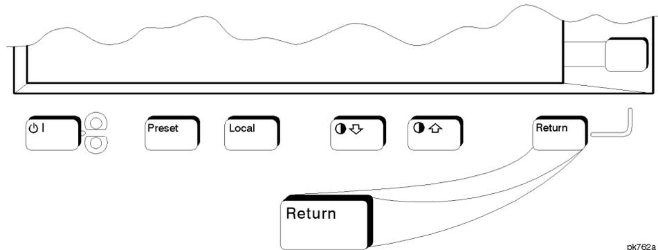
This front panel hardkey moves you from your current softkey menu to the softkey menu that precedes it. For example, press the **LF Out** front panel hardkey. The LF Out menu is displayed. Now press the **LF Out Source** softkey. (The arrow indicates that pressing this softkey will display another menu.) You should now see the LF Out Source menu. Press **Return**, and you are moved back to the LF Out menu.
