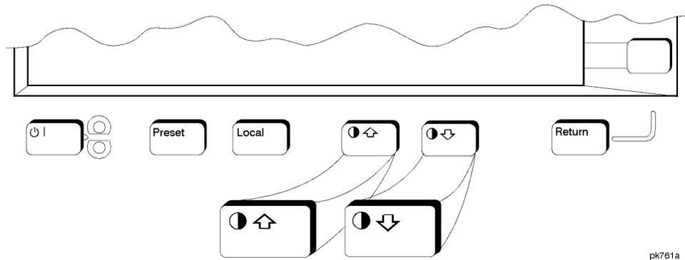
You can adjust the contrast of the display by pressing the decrease contrast key
