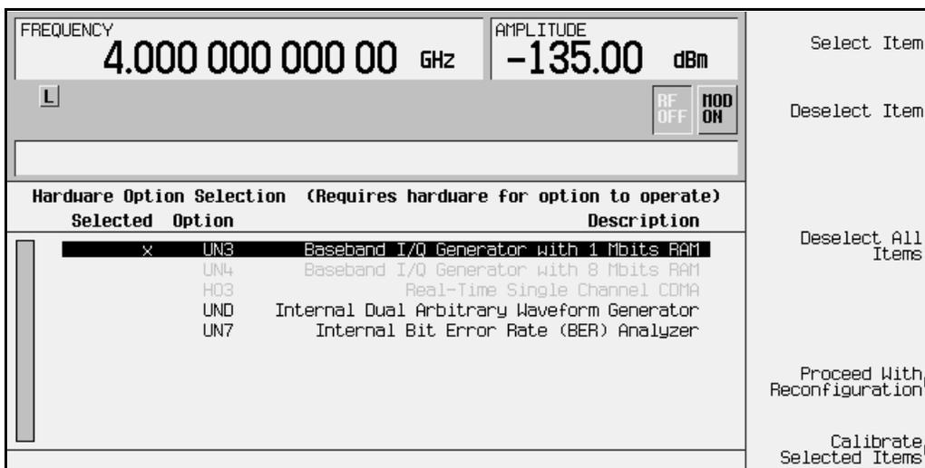
The display indicates which options are currently enabled for the signal generator. In this case Option UN3 is enabled, as indicated by the X placed in the “Selected” column.
