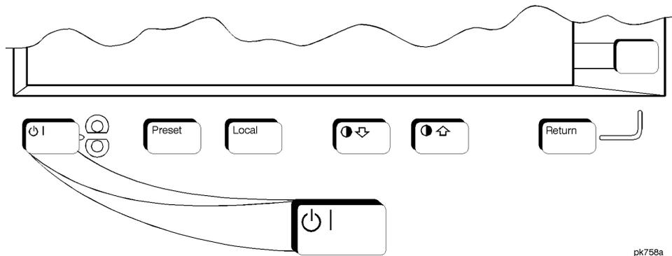
Pressing this front panel key toggles power to the signal generator either on (green LED on) or to standby (yellow LED on). In standby mode, the power switch is off but the instrument is still connected to the mains circuit by way of the power cord. The detachable power cord is the instrument disconnecting device. The front panel power switch, therefore, is not, and should not be used as, a line switch.
