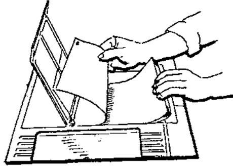
1 Remove Z-fold paper from package and open the paper compartment door on the top of the housing.
