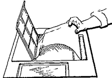
2 Place the new stack of paper into the compartment as shown in Fig.3.1; make sure the larger one of the two queuing holes is to the top of the unit.
