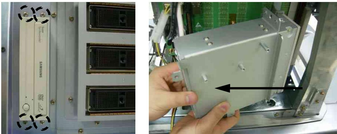
Figure 8-129 Unscrew 4screws and remove the DVD Assy
