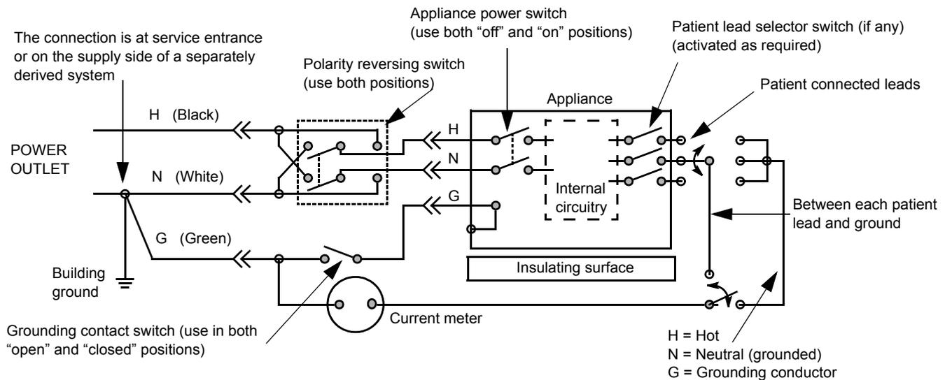
**Figure 10-7 Test Circuit for Measuring Non-Isolated Patient Leads**
