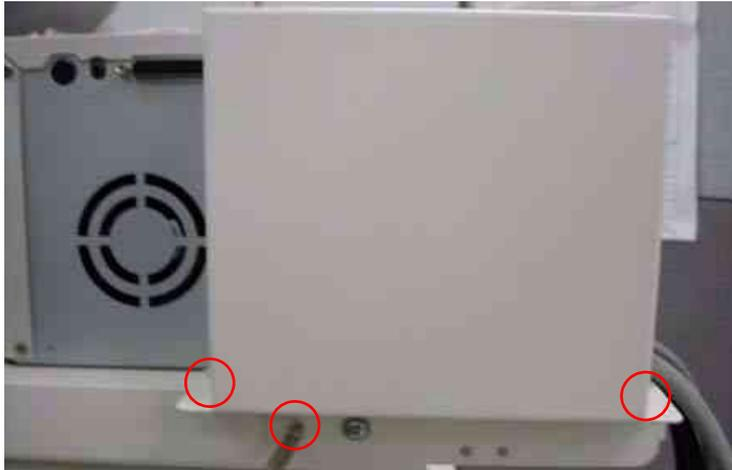
**Figure 8-281 Printer VCR DVD Fixture Top installation**
