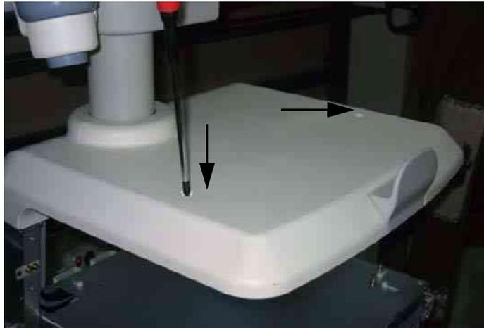
Figure 8-268 Color Printer Fixture Top Installation
