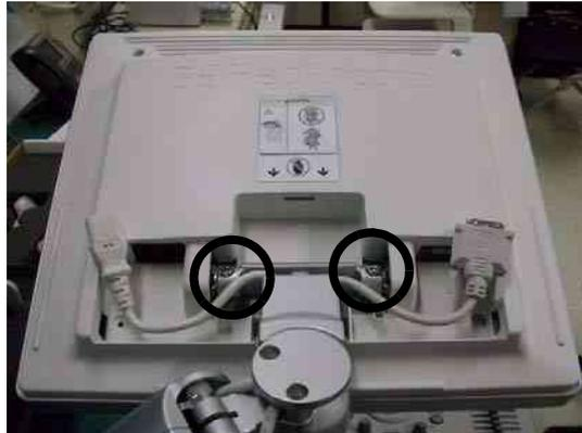
**Figure 8-16 Removing Spring**
