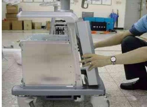
**Figure 8-90 Removal of front cover**
