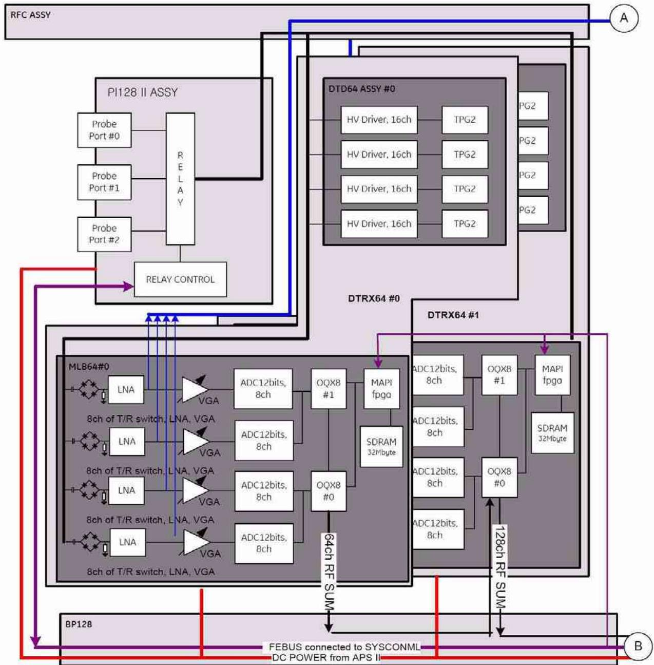
Figure 5-2 LOGIQ™ P6 Front End Block Diagram
