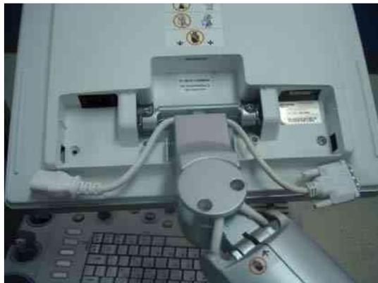
Figure 8-14 Removing the LCD Cable Cover
