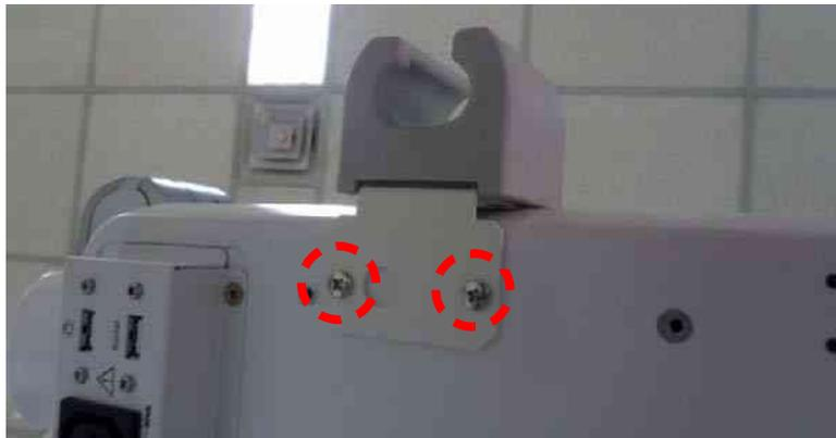
Figure 8-320 MTZ PROBE HOLDER Installation
