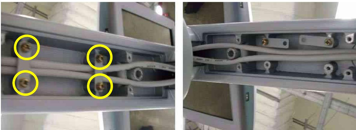
Figure 8-30 Unscrewing 4 screws
