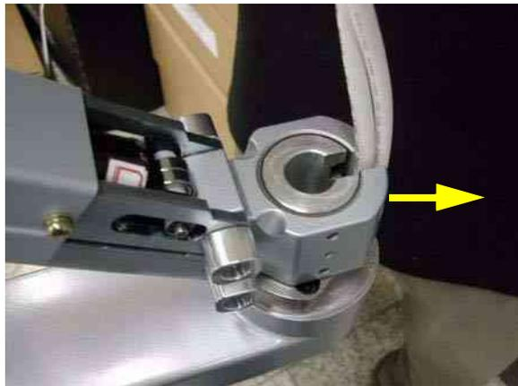
Figure 8-29 Pulling out power cable & DVI cable
