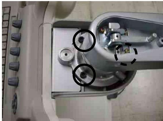
Figure 8-41 Assembling the arm neck pipe
