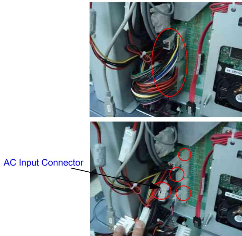
**Figure 8-103 APS II Connectors of backplane**
