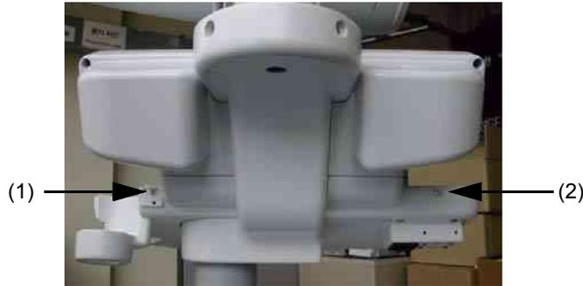
**Figure 8-72 Unscrews 2 screws**
