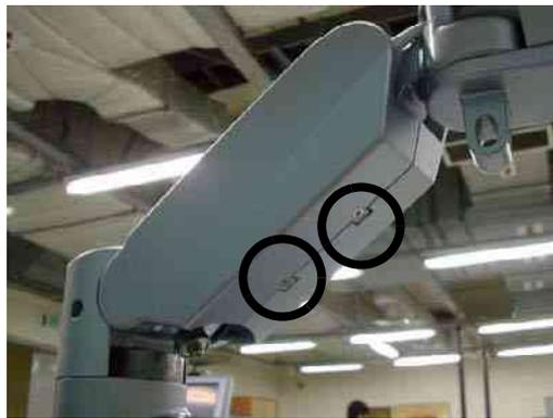
Figure 8-59 Assembling the Arm Cover L & R
