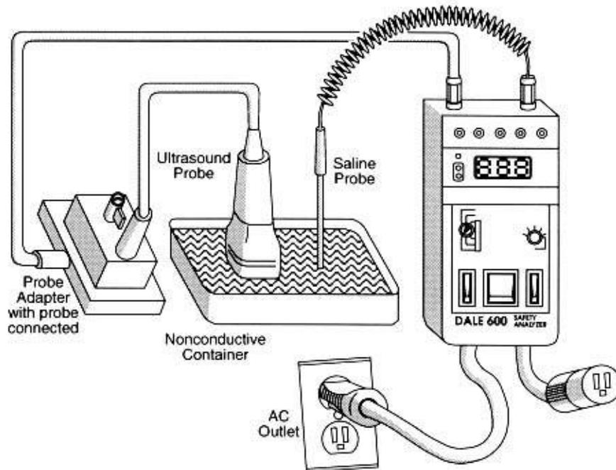
**Figure 10-10 Transducer Source Leakage Current Test**
