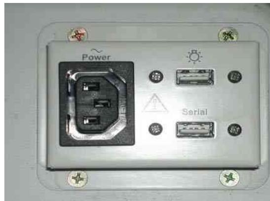
Figure 8-178 USB Port - OP Printer Bracket Back Panel
