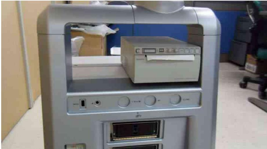
**Figure 8-237 BT11 BW PRINTER Option Installation**
