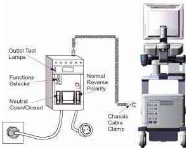
**Figure 10-6 Ground and Chassis Leakage Current Test**
