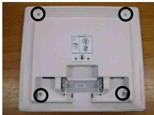
Figure 8-10 Removing the rear cover
