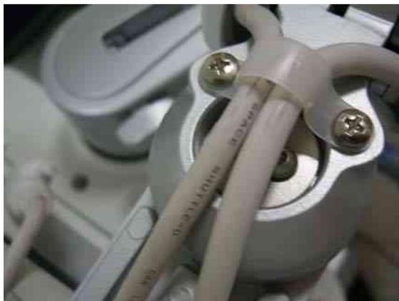
**Figure 8-50 Assembling the Cable clamp**
