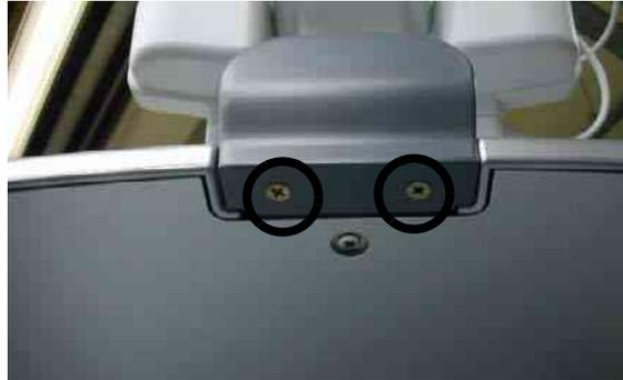
Figure 8-122 Screws on rear hook
