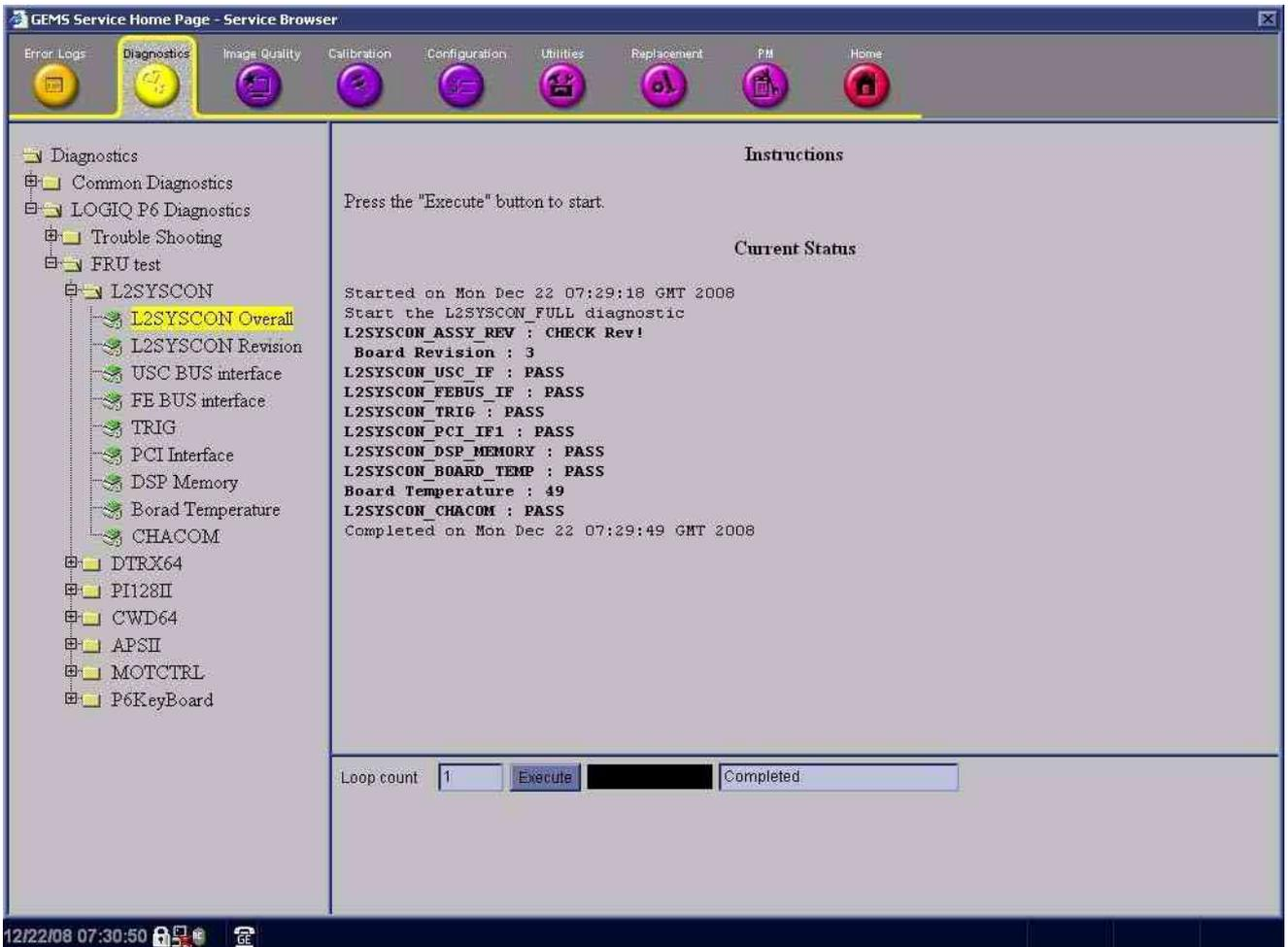
Figure 4-44 L2SYSCON Diagnostic Test
