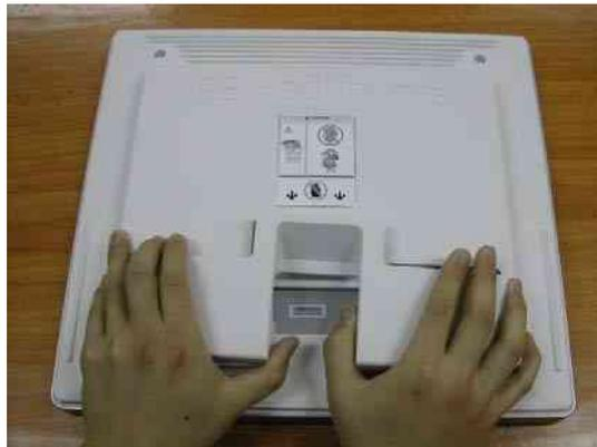
Figure 8-9 Removing the LCD Cable cover
