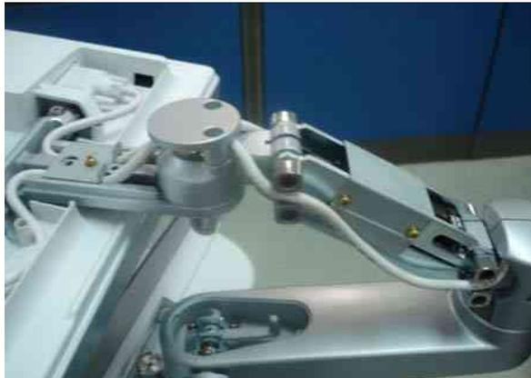
**Figure 8-48 Placing the Cables**
