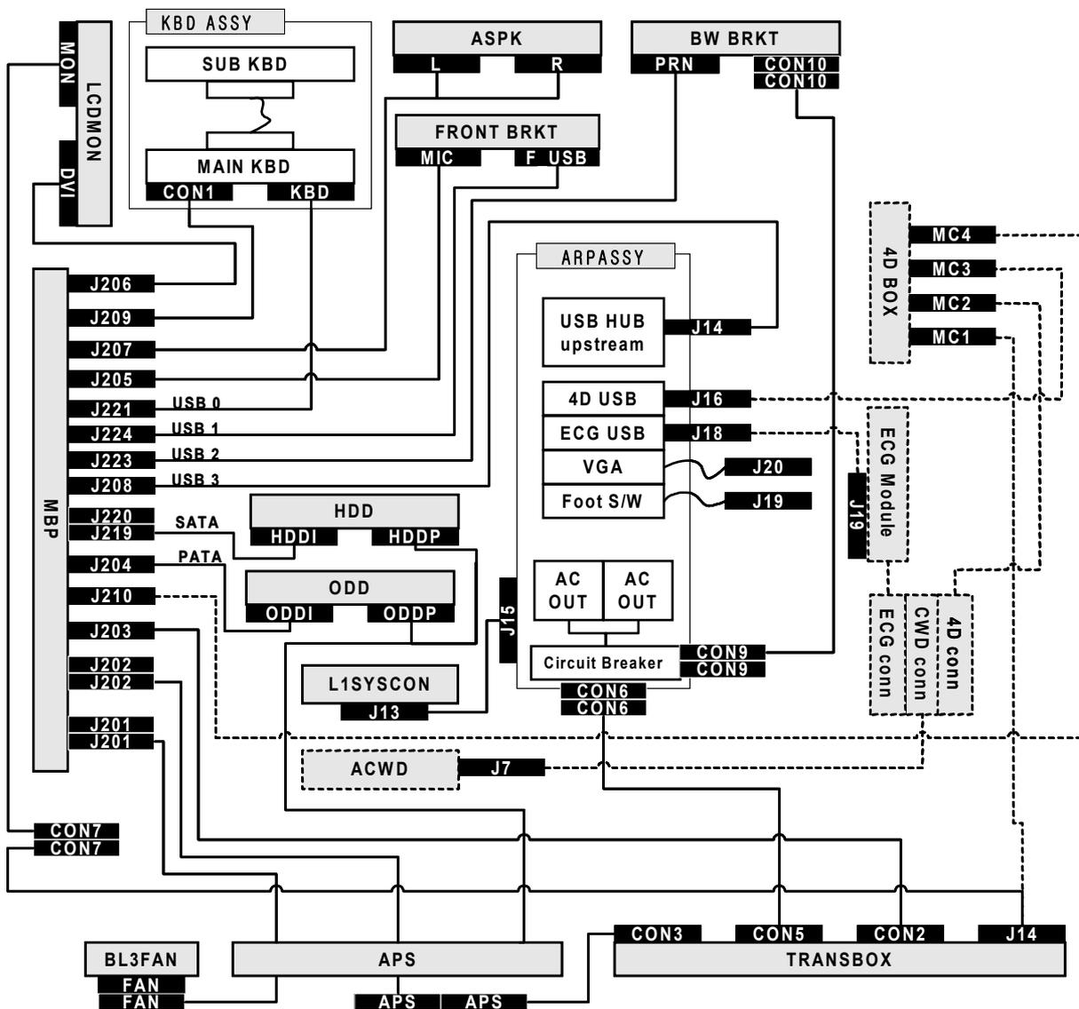
Figure 5-17 Cable Connection - Internal
