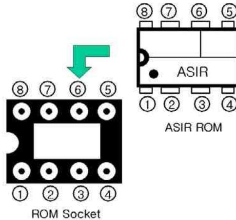
Figure 8-115 ASIR ROM mounting direction
