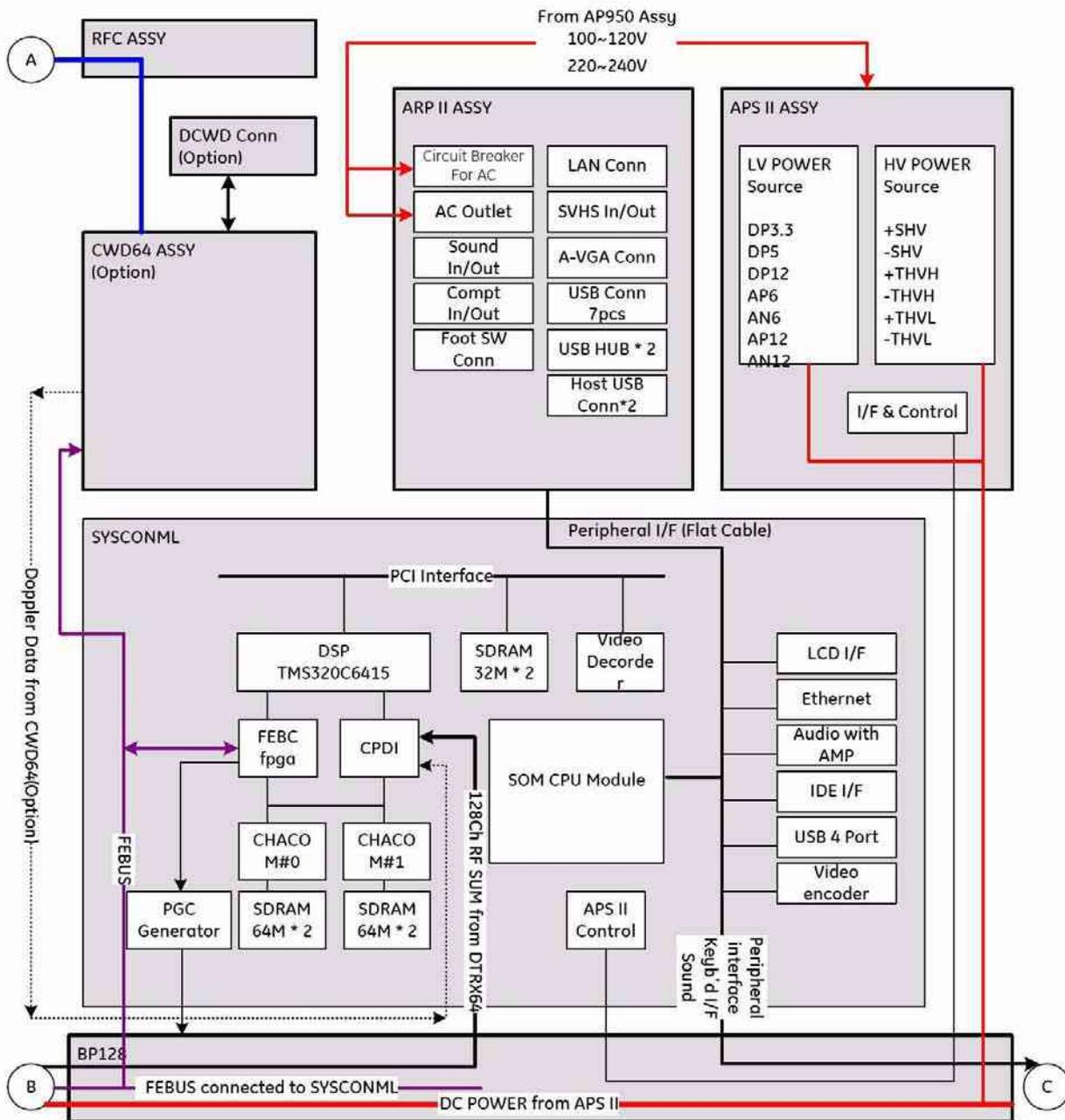
Figure 5-3 LOGIQ™ P6 Backend Block Diagram
