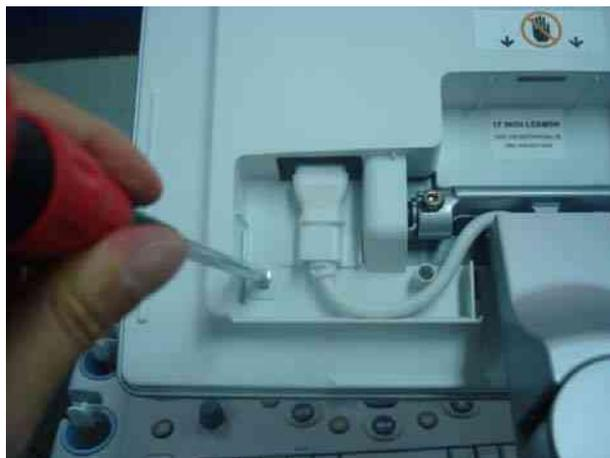
Figure 8-2 Removing the power cord bracket
