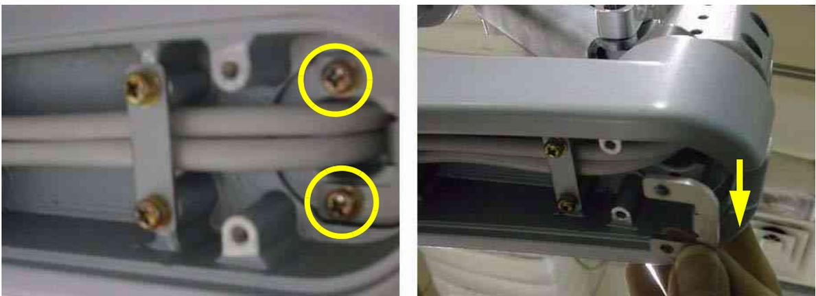
**Figure 8-27 Removing the Lower arm guide bracket**
