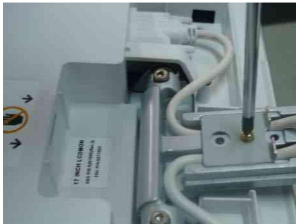
**Figure 8-49 Assembling the Cable bracket**
