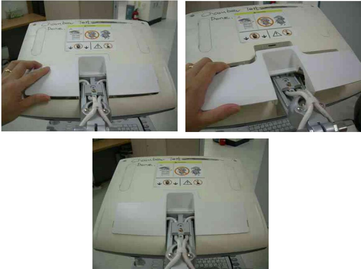
Figure 8-53 Assembling the LCD cable cover
