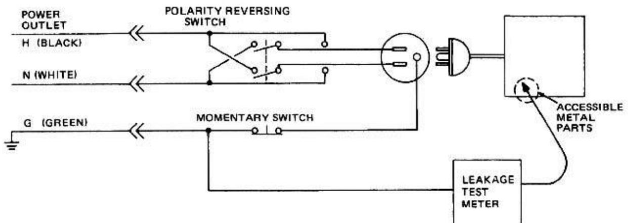
**Figure 10-5 Set Up for Chassis Source Leakage Current, IEC 601-1 Clause 19 - Continuous Leakage Currents and Patient, Auxiliary Currents**
