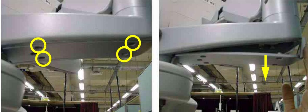
**Figure 8-64 Removing the Arm bottom cover**
