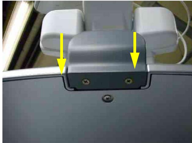
Figure 8-302 Rear Handle Installation
