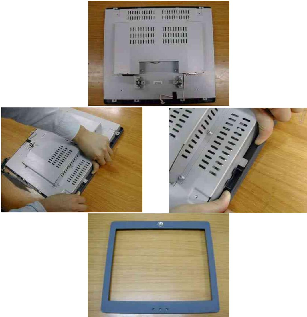
**Figure 8-8 Removing the 17" LCD front cover**
