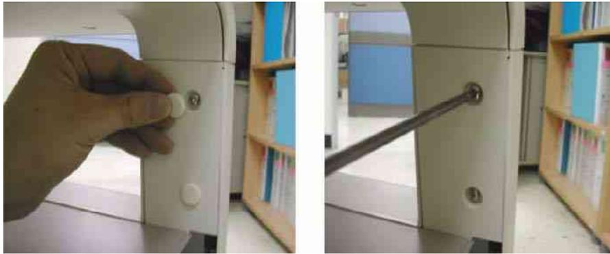
Figure 8-88 Screws of Dummy Cover
