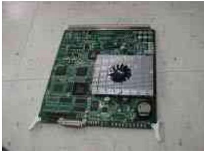
(a) Cooling Fan on L2 SYSCON II(SYSCONML)
