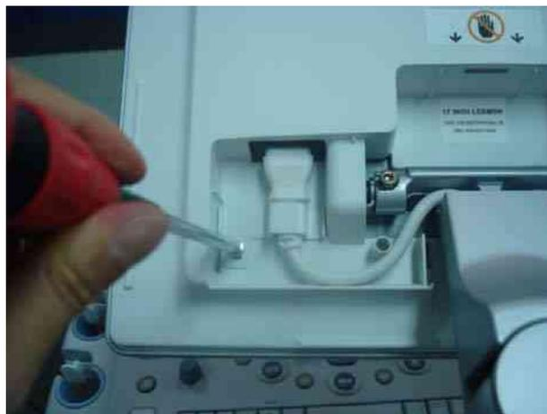
Figure 8-18 Removing the power cord bracket
