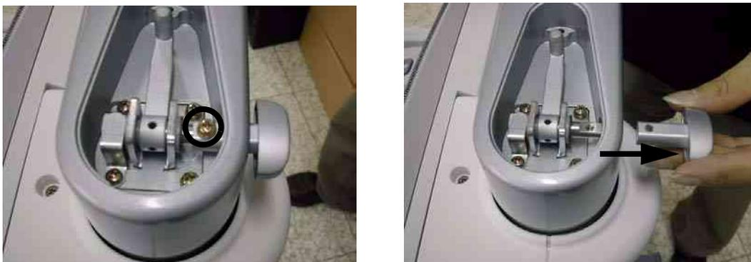
**Figure 8-68 Removing the Arm lock Knob**
