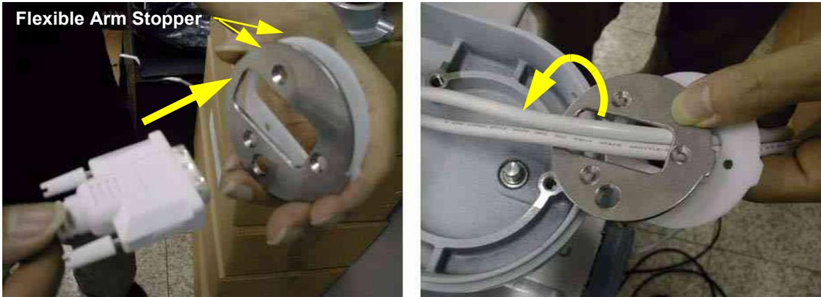
**Figure 8-36 Inserting cables to the flexible arm stopper**
