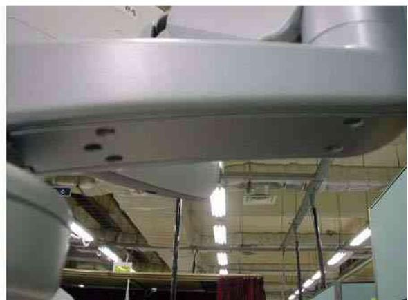
Figure 8-60 Assembling the Arm bottom cover
