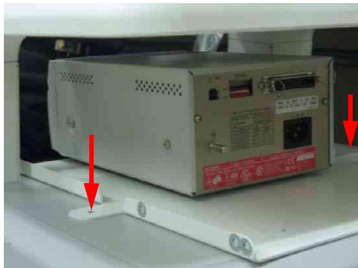
**Figure 8-249 BW Printer Fixture Middle installation**
