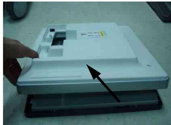
**Figure 8-5 Removing the 17" LCD rear cover**
