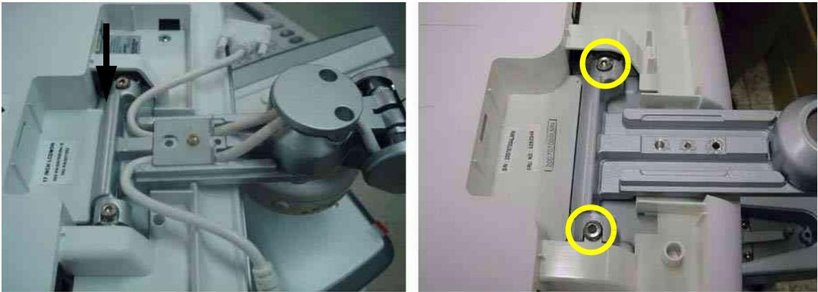
**Figure 8-42 Screwing 2 screws**
