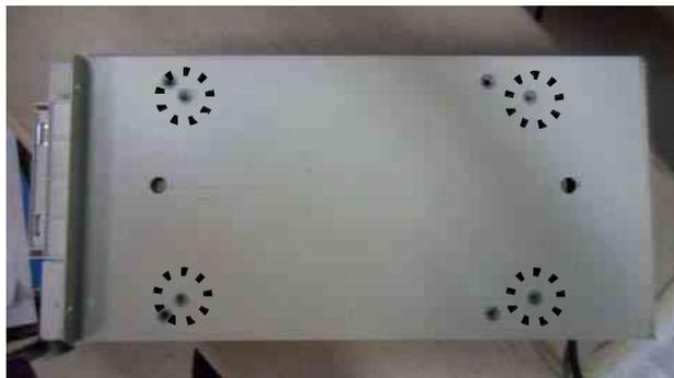
Figure 8-272 Color Printer Fixture Top Installation
