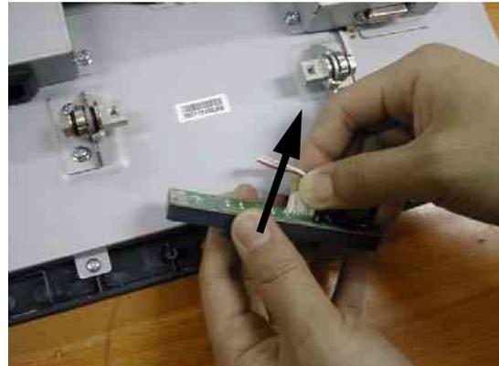
**Figure 8-6 Separating the OSD key assy**
