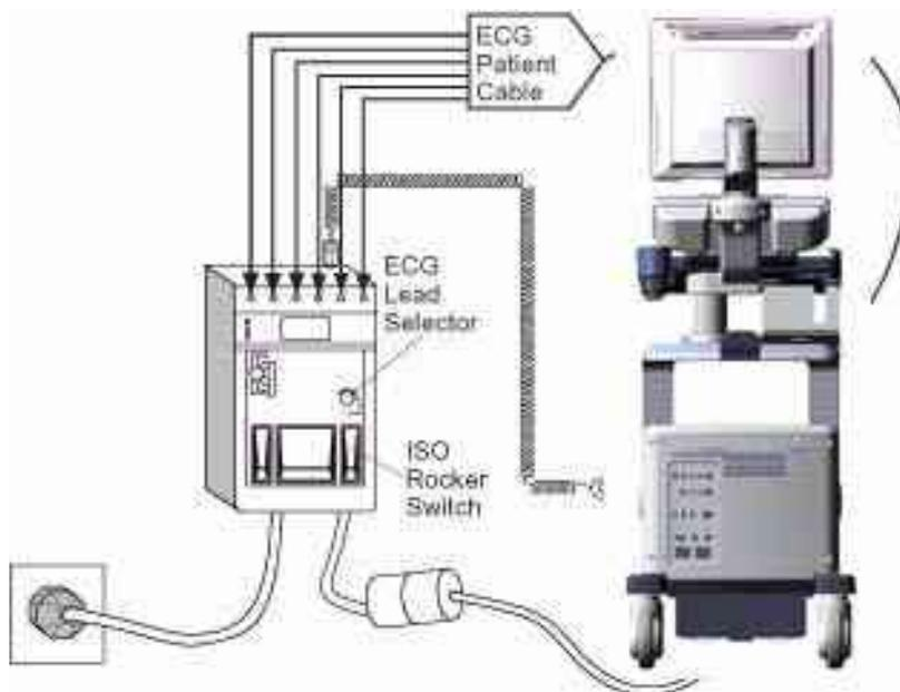
**Figure 10-8 ECG Leakage Current Test**
