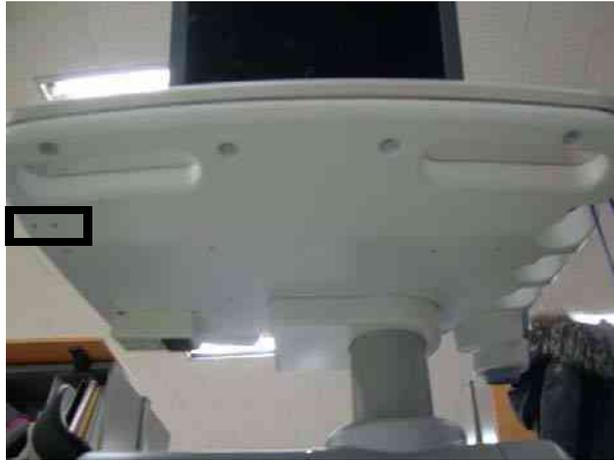
Figure 8-232 Microphone option holes
