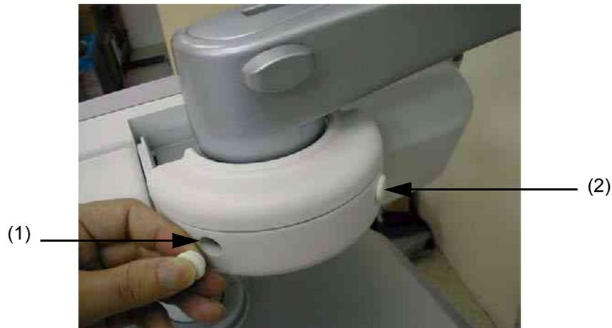
Figure 8-98 rubber cap of neck rear cover
