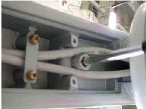
**Figure 8-56 Assembling the Lock Cover**
