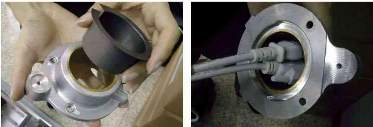
**Figure 8-37 Inserting the oilless bush**
