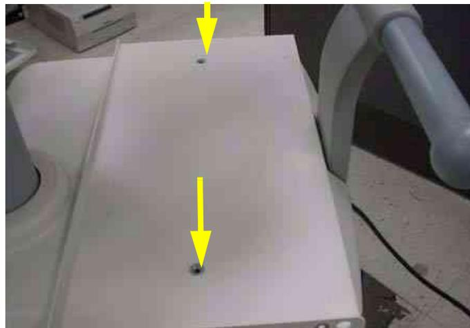
Figure 8-264 Printer VCR DVD Fixture installation top
