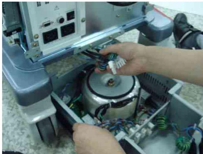
**Figure 8-145 Insert the Transbox assy**
