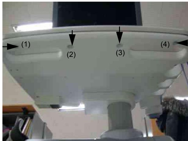
Figure 8-71 Unscrews 4 screws
