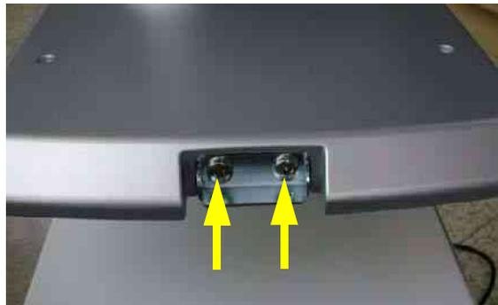
Figure 8-123 Screws on the rear hook fix brkt
