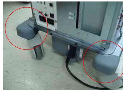
Figure 8-312 Protect Cover Installation
