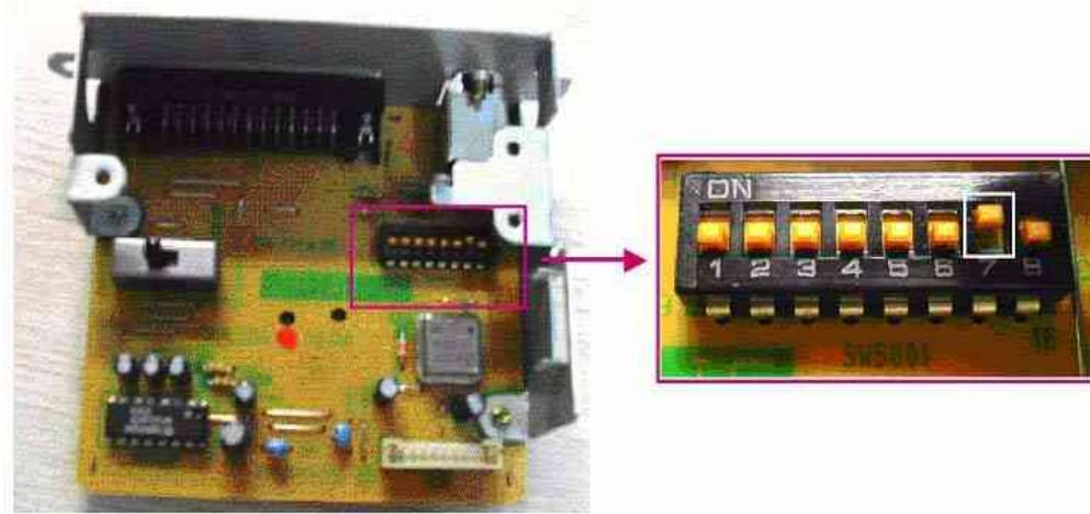
Figure 8-284 DIP Switch on the Panel
