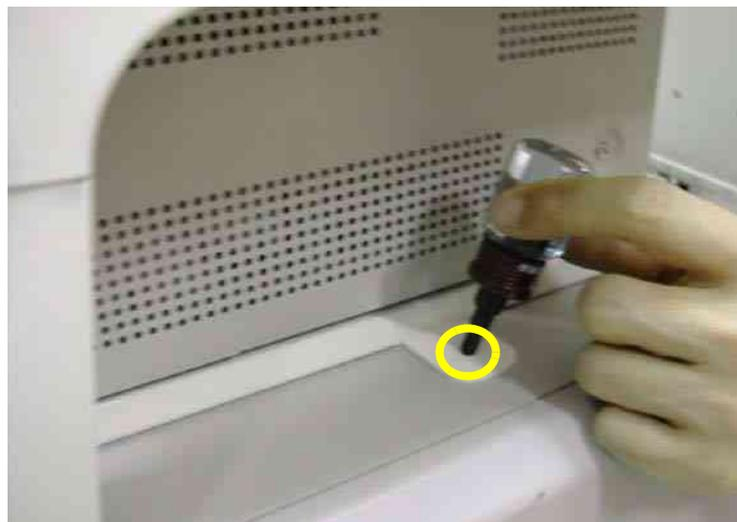
**Figure 8-259 Color Printer Fixture Middle installation**
