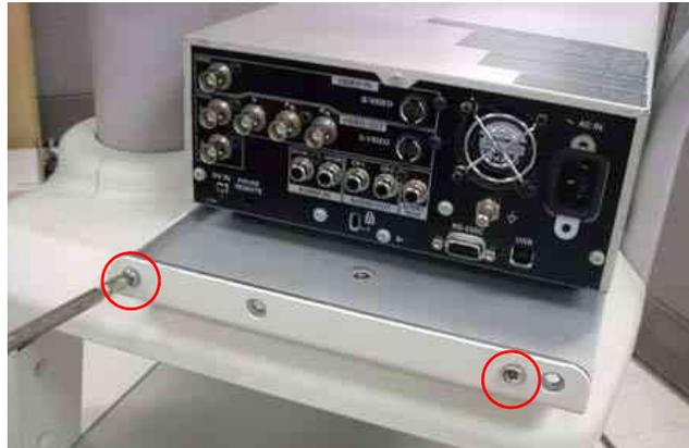
**Figure 8-298 Printer VCR DVD Fixture Top installation (LQ MD800)**
