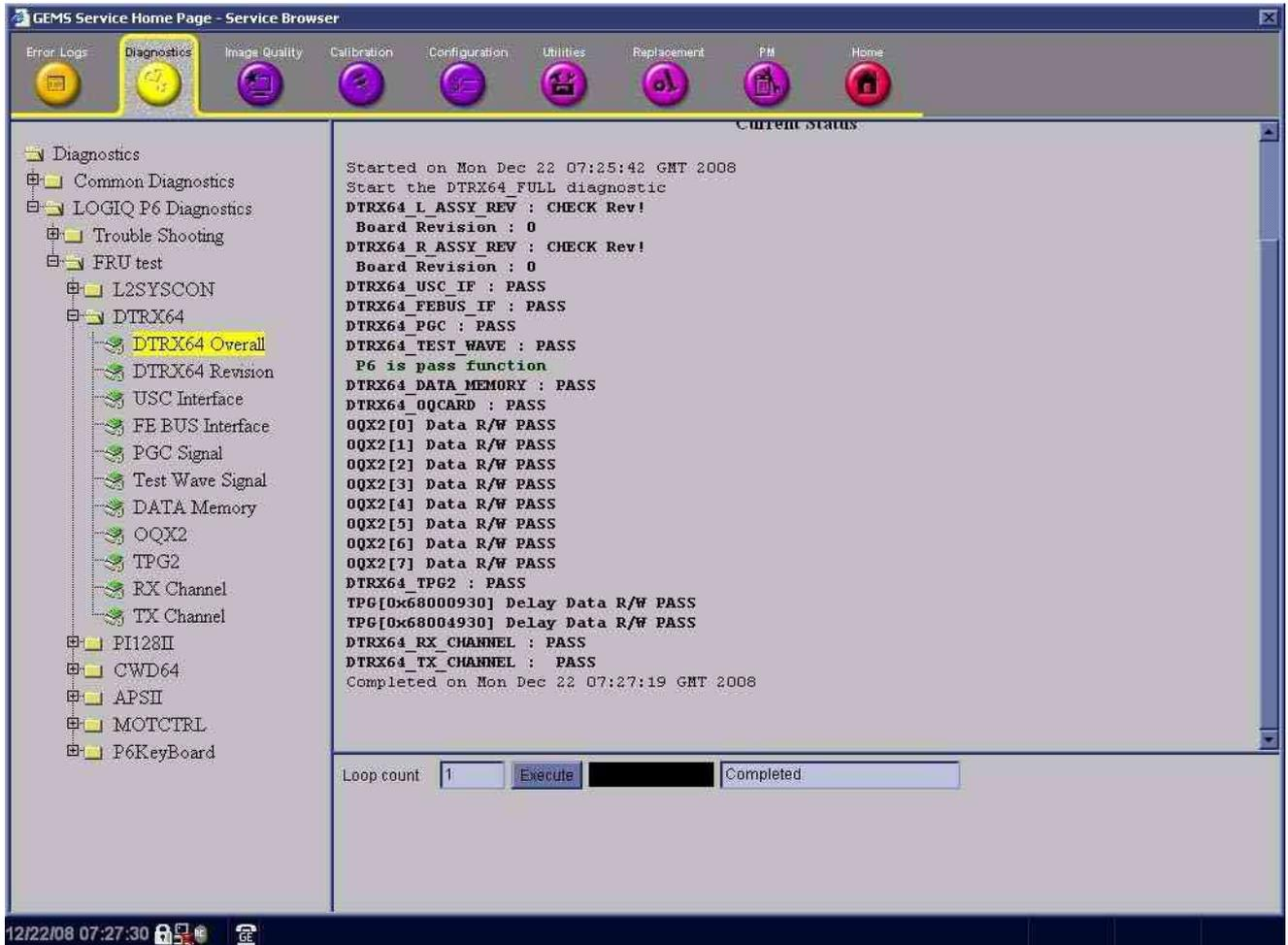
Figure 4-36 DTRX64II Diagnostic test
