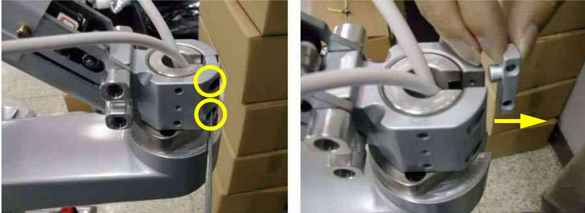
Figure 8-28 Removing the Arm stopper
