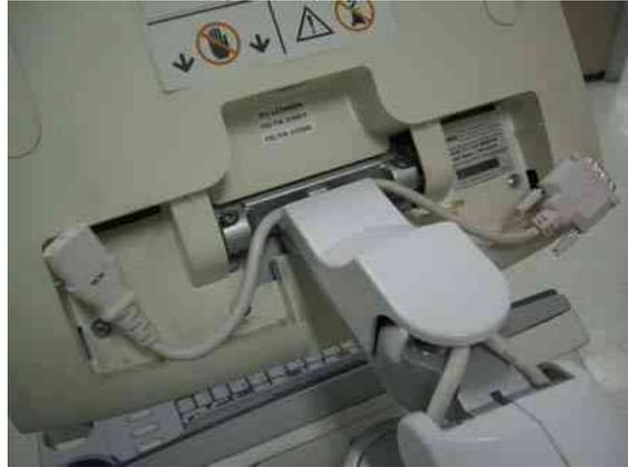
**Figure 8-3 Disconnecting power cable and DVI cable**
