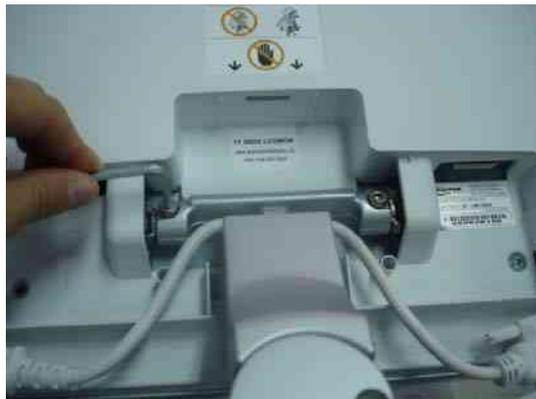
Figure 8-15 Removing the power code bracket
