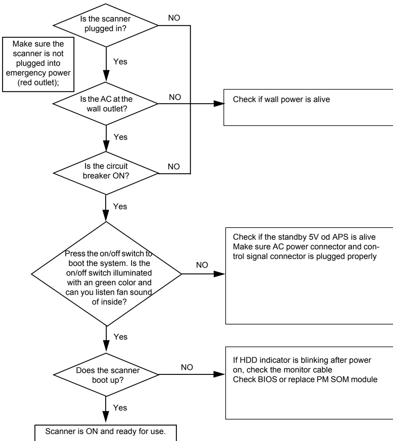
Figure 7-13 Power On / Boot Up Flowchart
