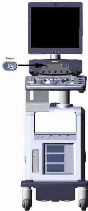
**Figure 3-9 Power On/Off Switch Location**
