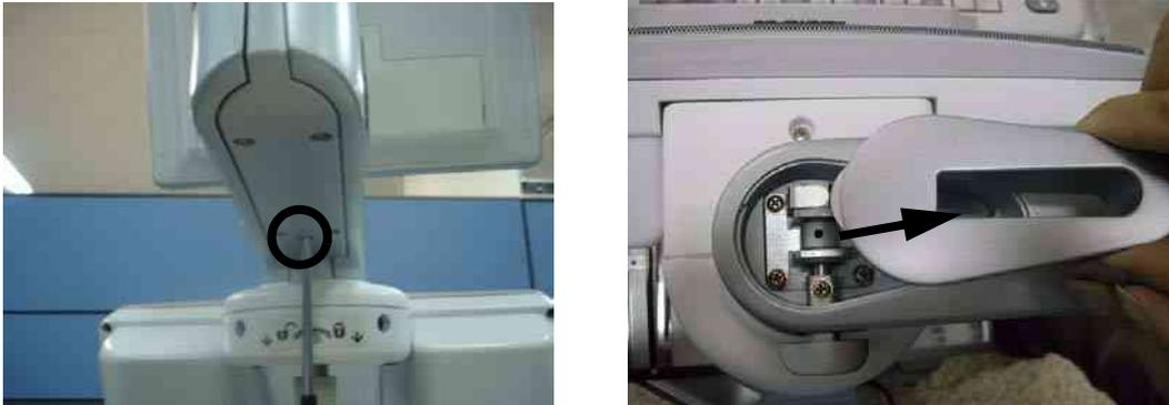
**Figure 8-66 Removing the Arm lock cover**
