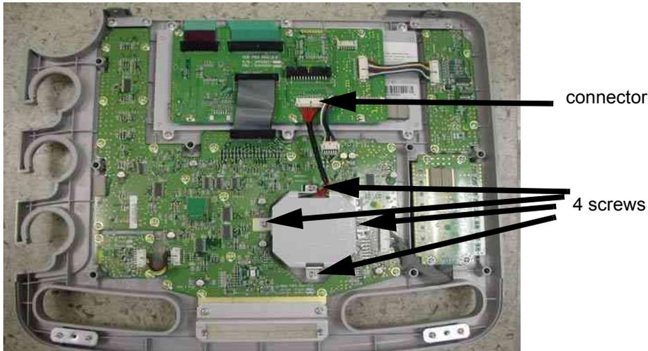
Figure 8-75 Screws and connector for Trackball
