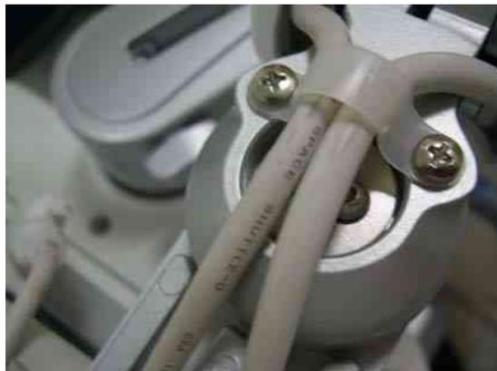
**Figure 8-21 Removing the Cable clamp**
