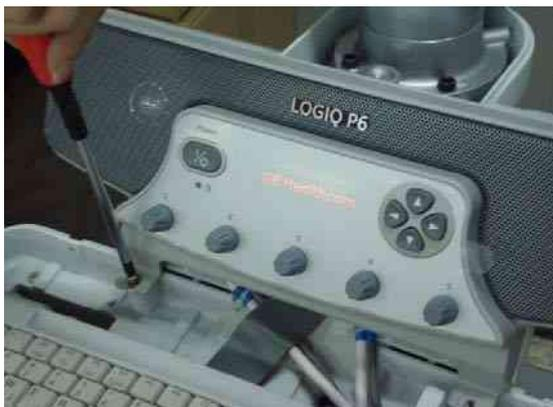
**Figure 8-74 4 Screw Sub Keyboard Assy**
