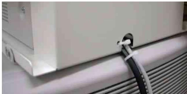
Figure 8-257 Color Printer Fixture Middle installation
