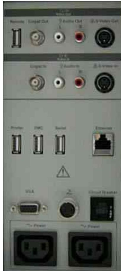
Figure 3-14 Rear Connector Panel
