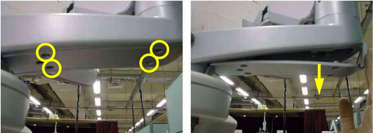
**Figure 8-25 Removing the Arm bottom cover**
