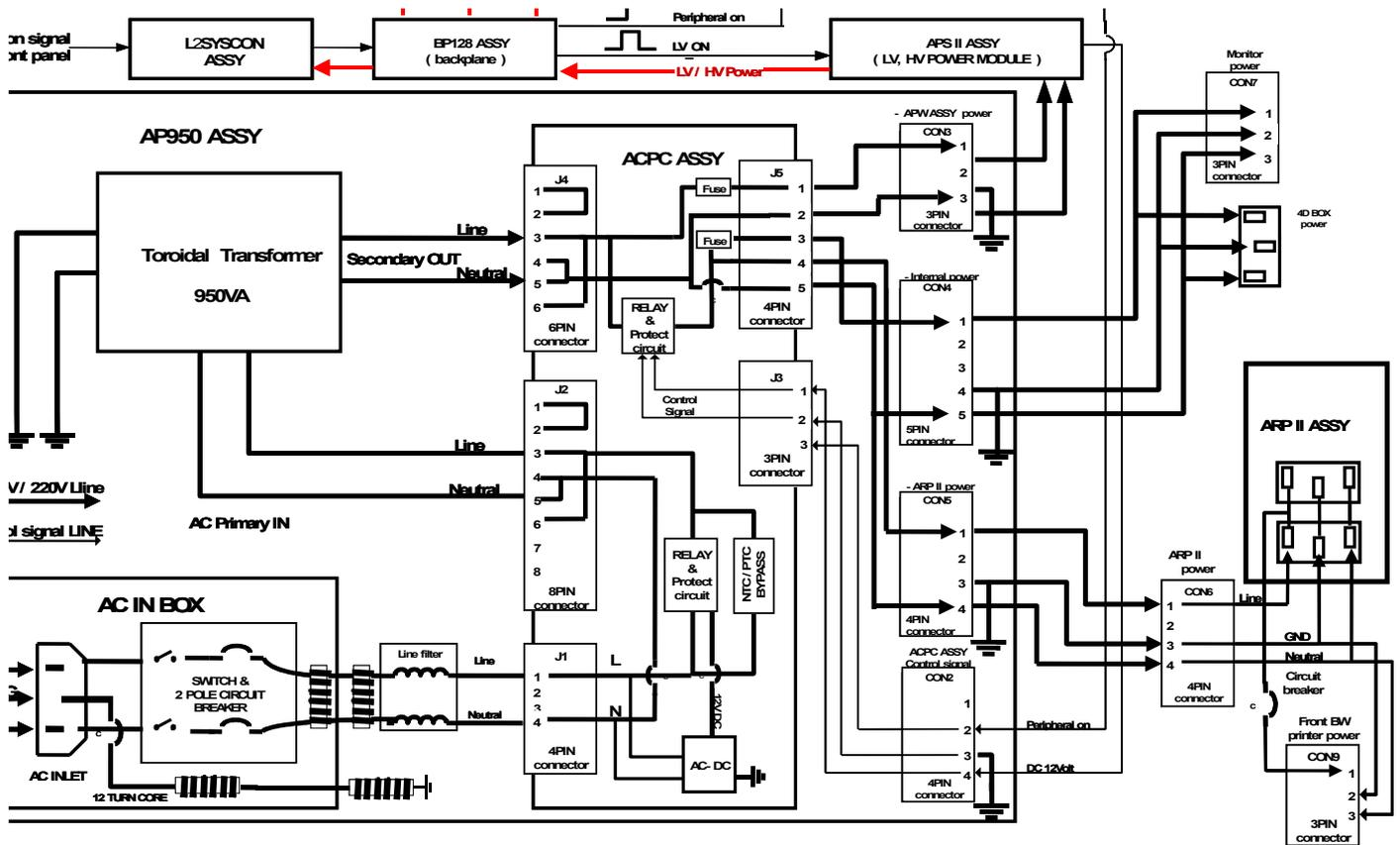
Figure 5-8 AC Power Assy Block Diagram
