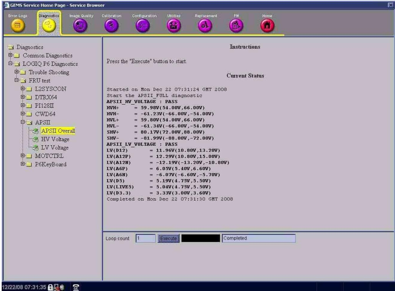
Figure 4-45 APS II Diagnostic Test
