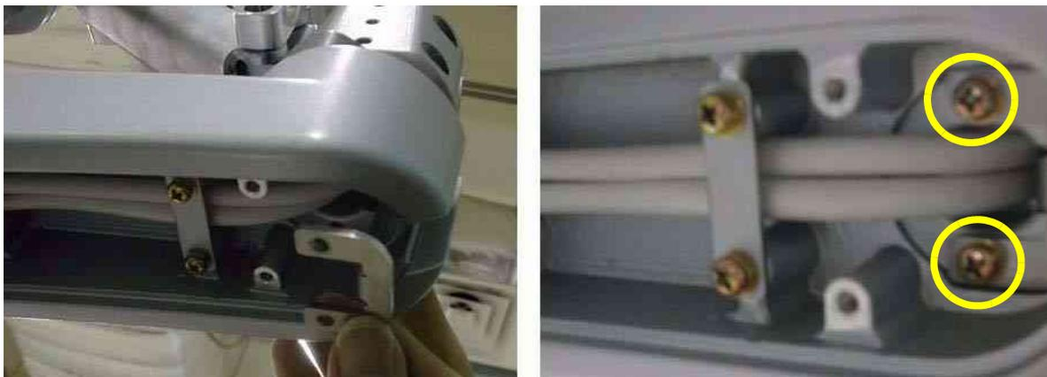
Figure 8-46 Assembling the Lower arm guide bracket
