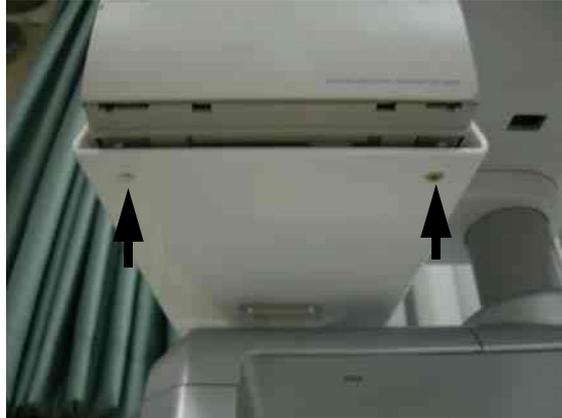
**Figure 8-245 BW Printer Fixture Keyboard installation**
