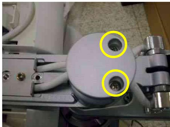
**Figure 8-65 Removing the Arm cable cover**
