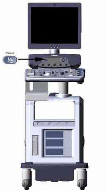
Figure 4-2 Power On/Off Standby Switch Location
