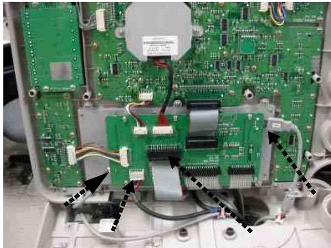
**Figure 8-73 Lifting the top cover & Disconnecting 5 Cables**
