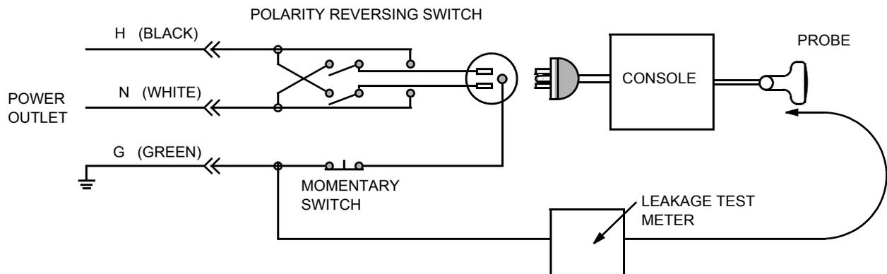
Figure 10-9 Set Up for Probe Leakage Current
