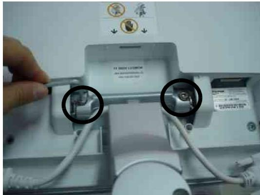
**Figure 8-4 Separating the 17" LCD monitor**
