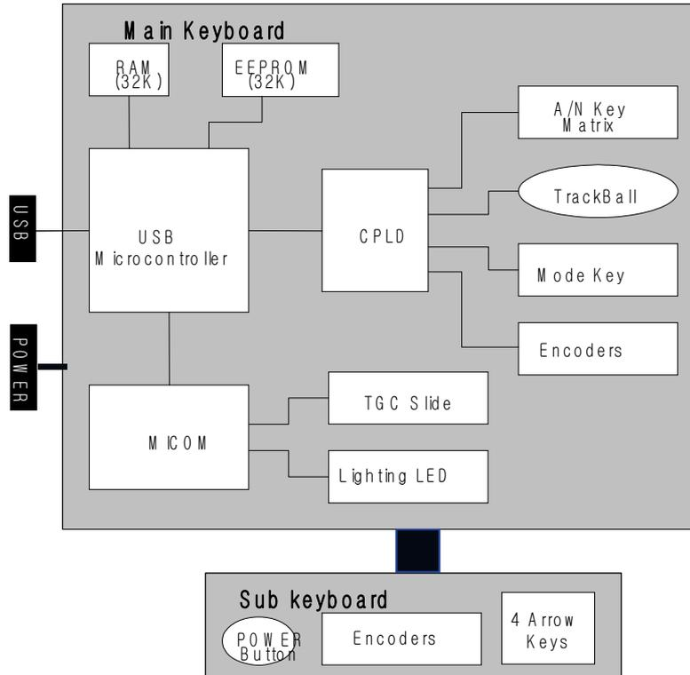
**Figure 5-10 Keyboard Block Diagram**
