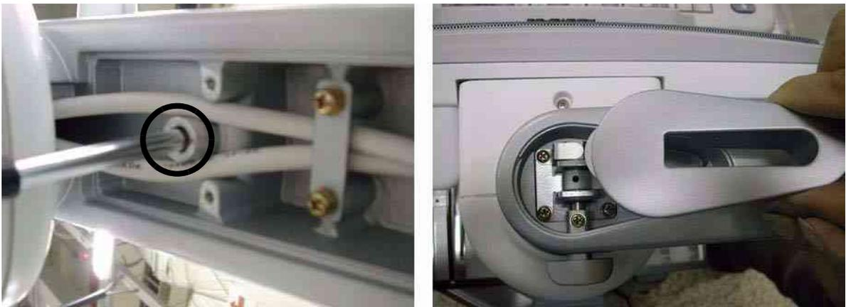
**Figure 8-26 Removing the Lock cover**
