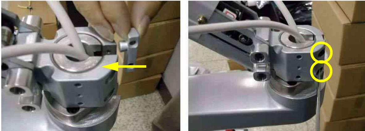
Figure 8-45 Installing the Arm stopper
