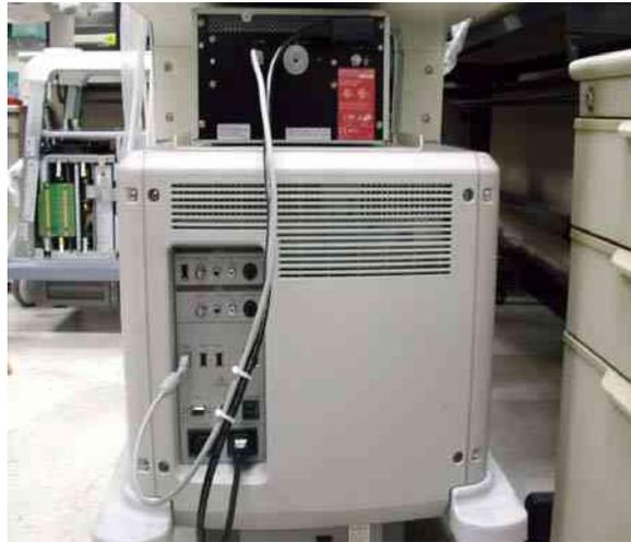
Figure 8-255 Color Printer Fixture Middle installation
