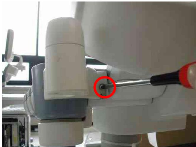
Figure 8-241 Cable Arm Hook installation
