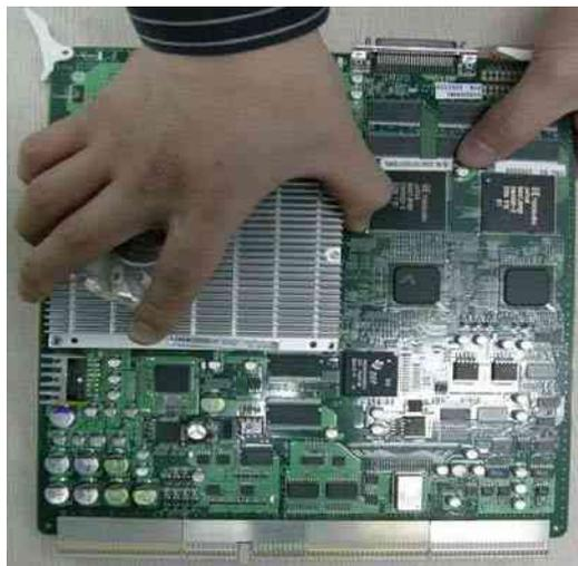
Figure 8-117 Remove a SOM from SYSCONML Assy
