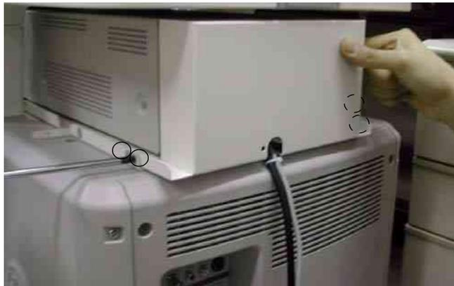
Figure 8-256 Color Printer Fixture Middle installation
