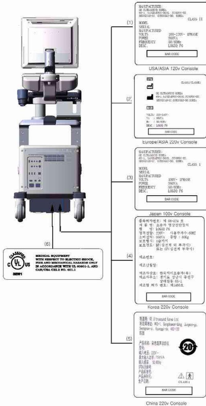
Figure 1-1 OUTSIDE MARKINGS OF LOGIQ™ P6/P6 Pro (Rear)
