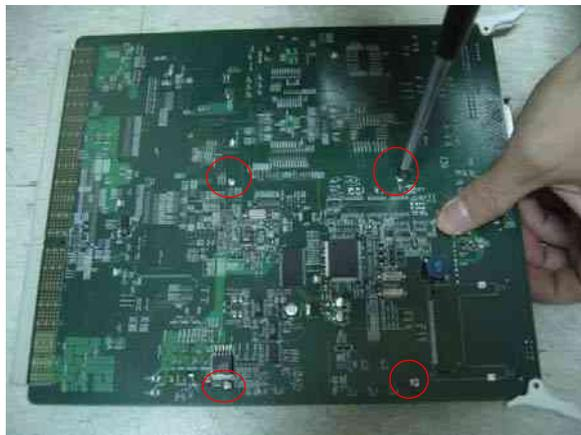
Figure 8-116 4 screws for SOM on SYSCON
