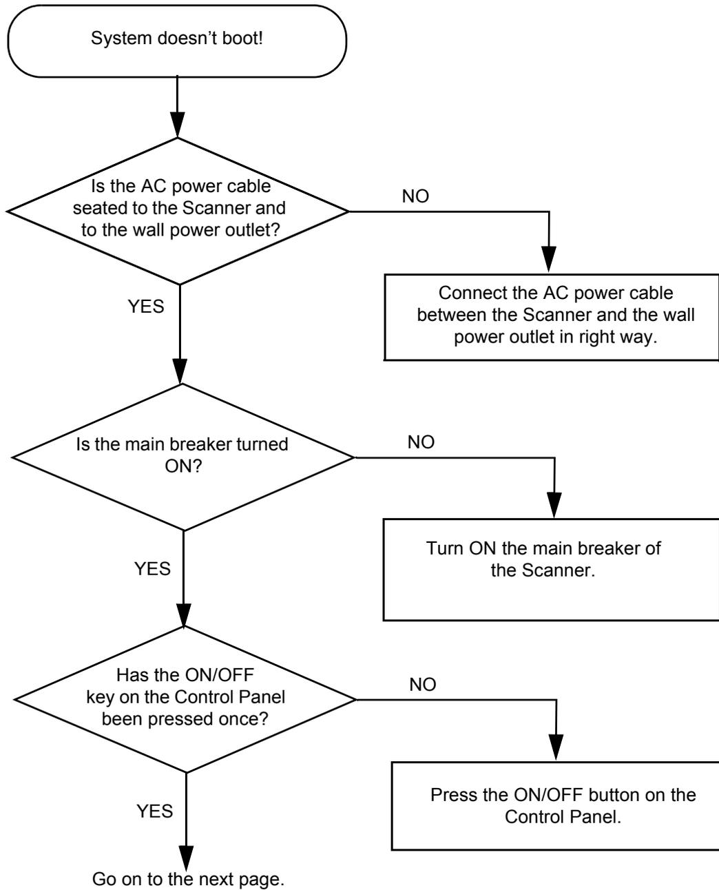
Figure 7-14 System does not Boot
