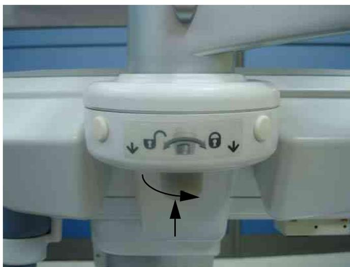
**Figure 6-3** Locking the Flexible LCD arm
