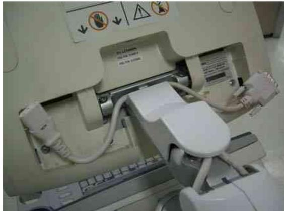
**Figure 8-19 Disconnecting power cable and DVI cable**
