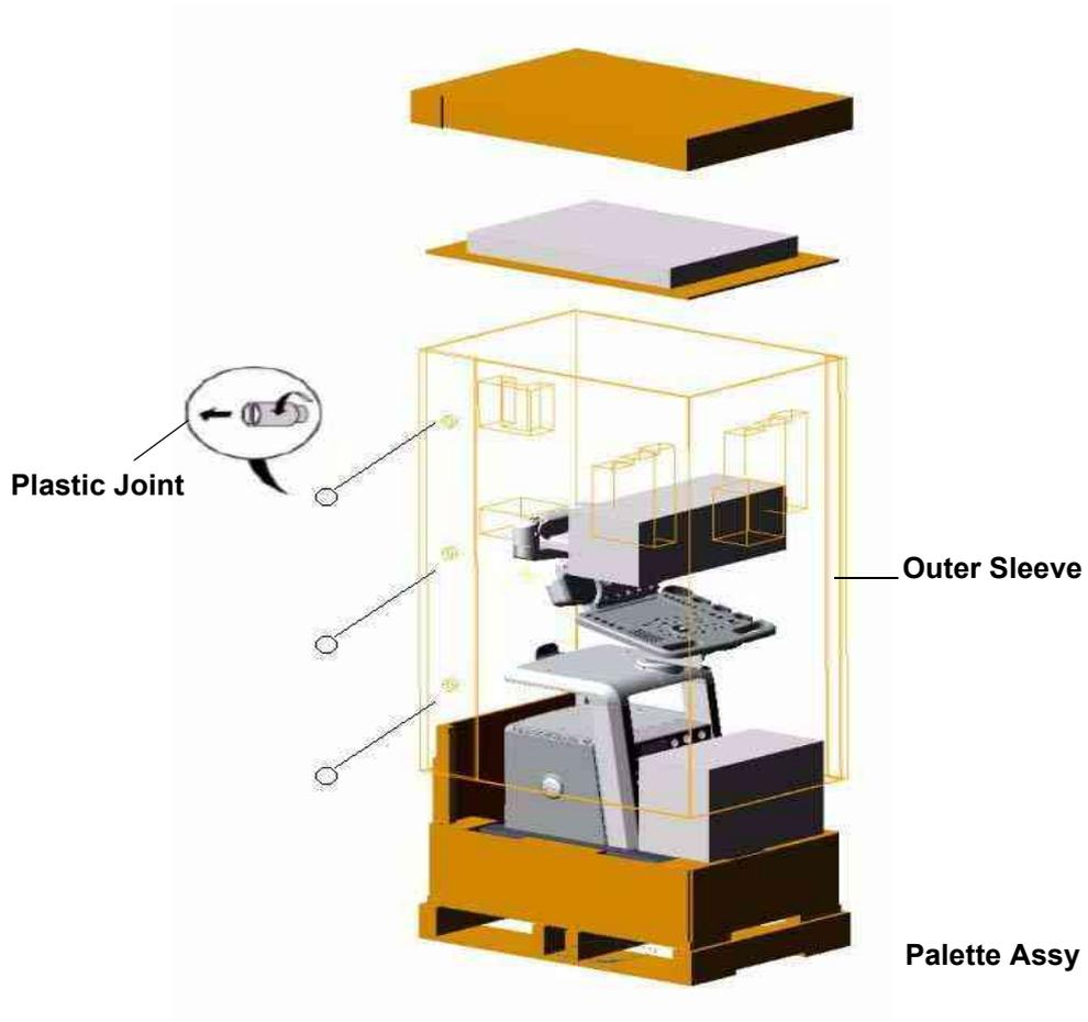
Figure 3-5 Removing Plastic Joints and Sleeves
