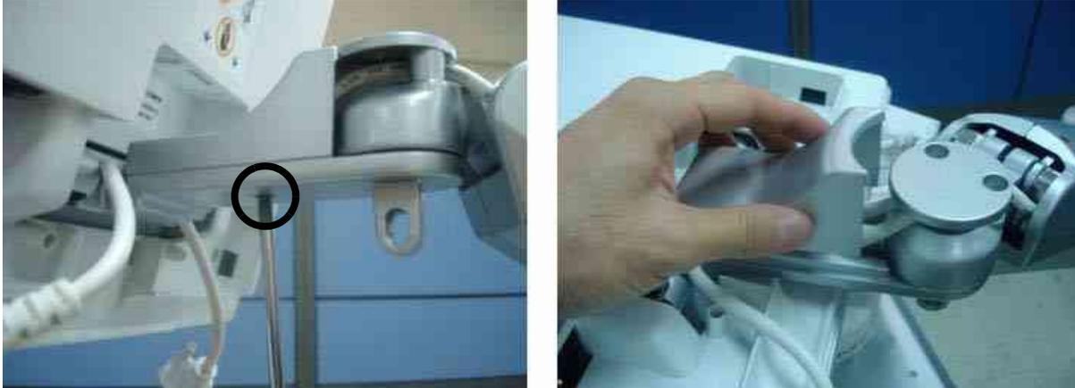
**Figure 8-69 Removing the Arm fold cover**
