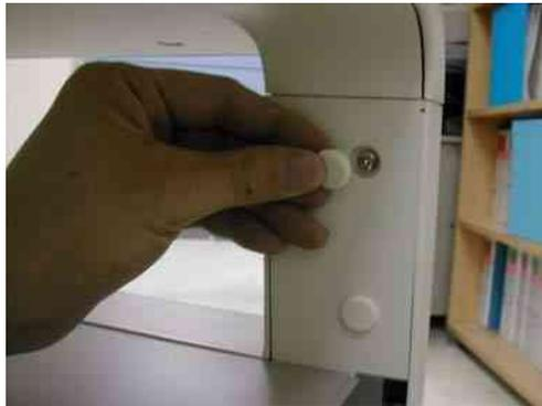
Figure 8-100 rubber cap of dummy cover
