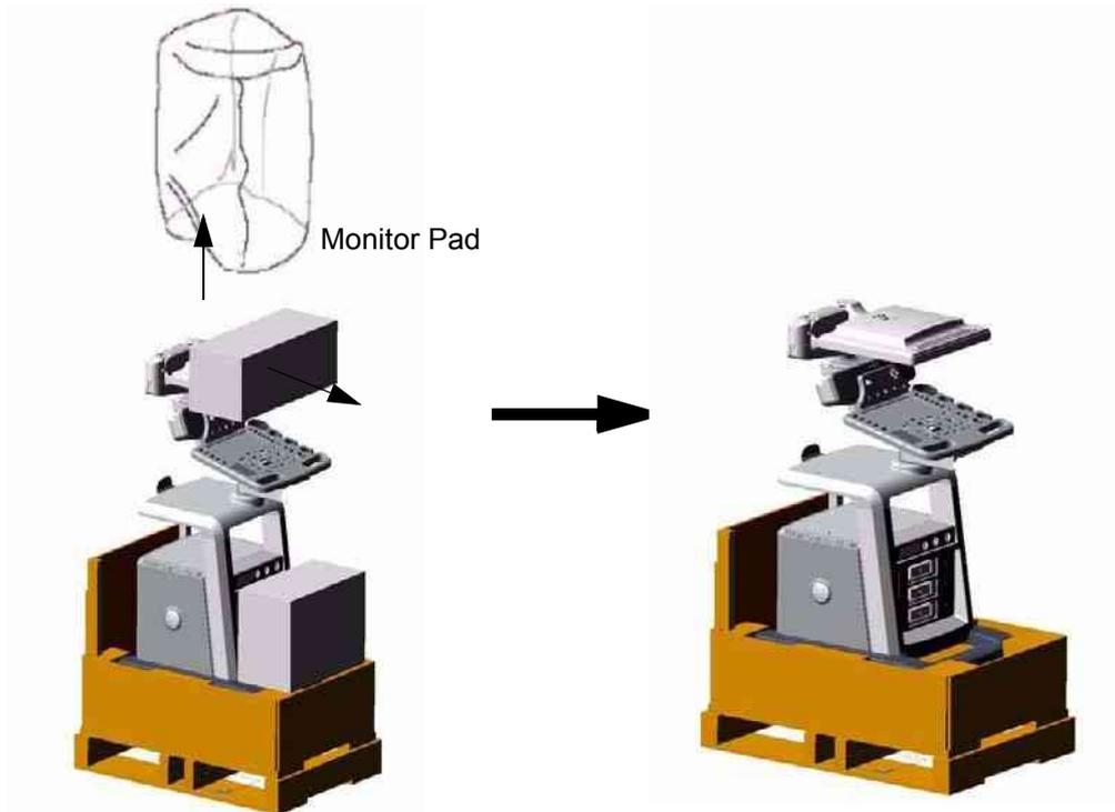
Figure 3-6 Moving the LOGIQ™ P6/P6 Pro from the crate
