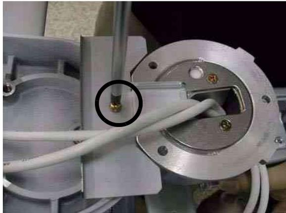
**Figure 8-33 Removing OP bracket**
