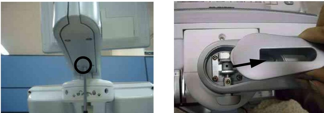
**Figure 8-67 Removing the Arm lock cover**
