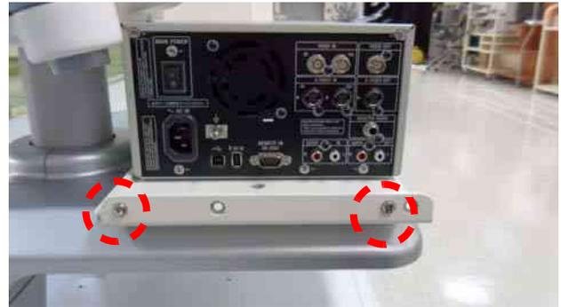
**Figure 8-325 SONY DVR Fixture Top Installation**
