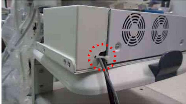
Figure 8-274 Color Printer Fixture Top Installation
