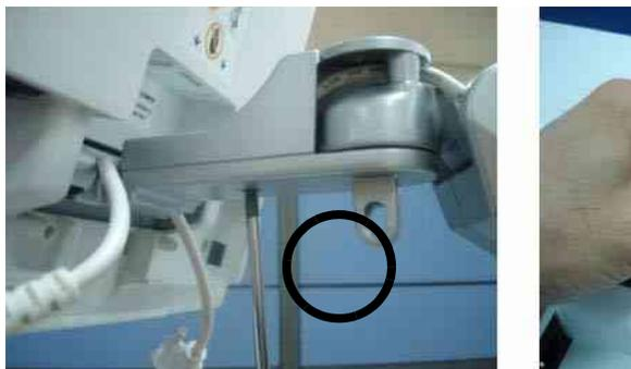
**Figure 8-20 Removing the Fold cover**
