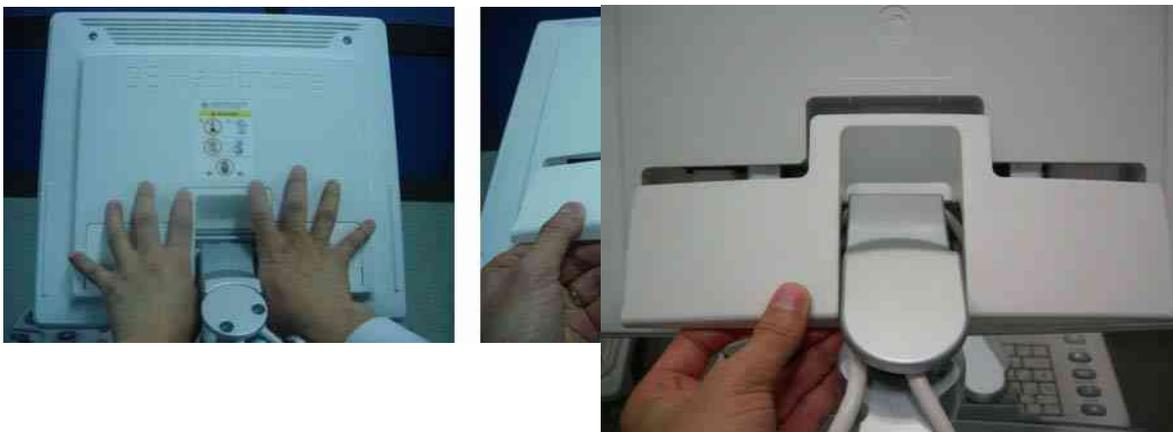
Figure 8-1 Removing the 17" LCD cable cover
