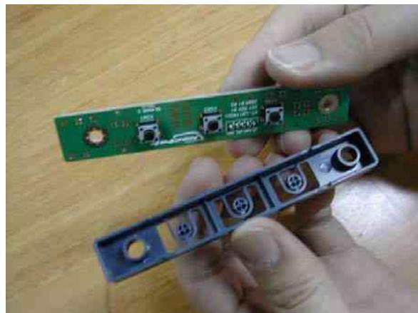
**Figure 8-7 Separating the 17" LCD tact knob**
