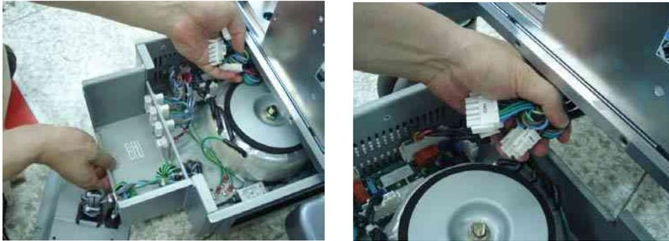
**Figure 8-144 Pull out the Transbox assy**
