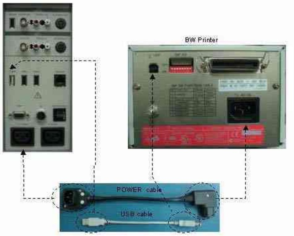
Figure 5-18 Digital BW Printer
