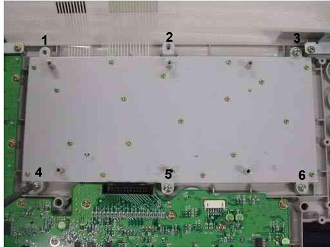
**Figure 8-78 Screws on the A/N Key**
