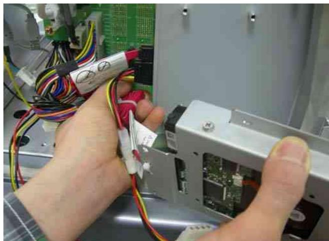
Figure 8-137 Disconnect the SATA Cable
