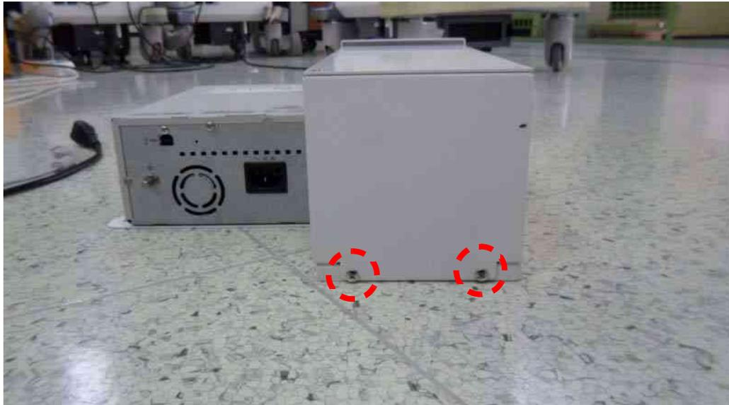
**Figure 8-315 BT11 Drawer Option Installation**
