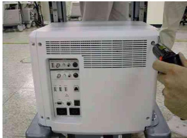
Figure 8-91 4 rubber caps and 4 screws on Rear Cover
