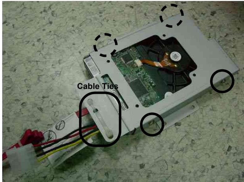
**Figure 8-138 Separate HDD and HDD Fixture Bracket**
