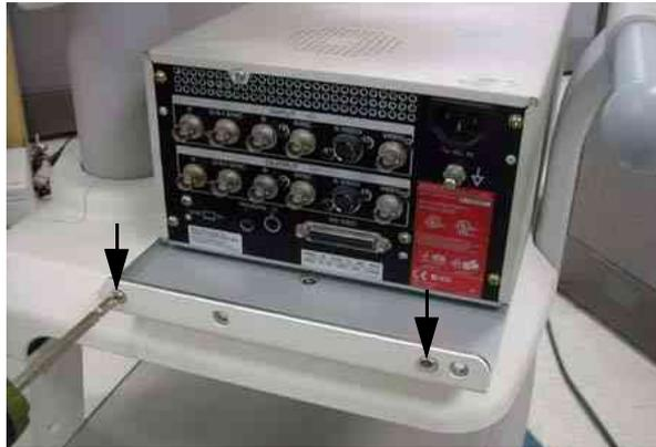
**Figure 8-266 Printer VCR DVD Fixture installation top**
