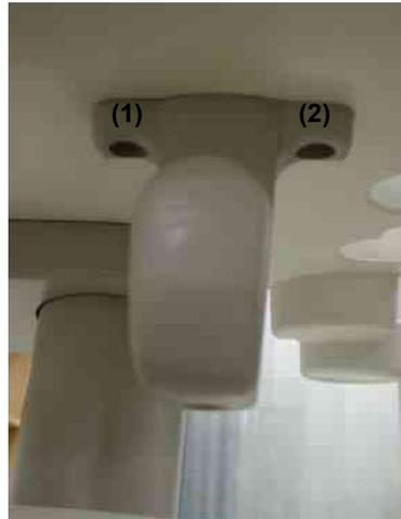
**Figure 8-126 Cable hook on the bottom of keyboard**
