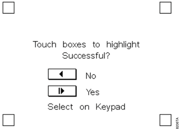
Figure 13. Confirmation screen for the Touch screen. Touch all four boxes; if they all change color, press the Stop/Run button on the instrument keypad. If they do not all change color, press the back arrow button and repeat the calibration and confirmation.
