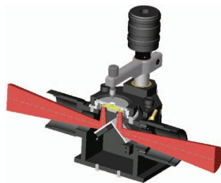
Figure 3. IR beam path for Pike ATR cell.
