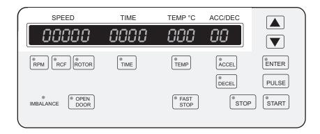
Digital displays indicate rotor speed, run time, rotor chamber temperature, and numbers that represent selected acceleration and deceleration profiles. When the power is turned on, they show the operating parameters of the most recent run performed before the power was turned off. The displays serve a dual purpose.
