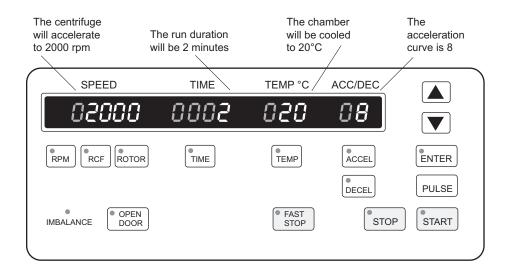
Figure 3-3. Default Parameters. The control panel shown is a refrigerated model; default values are the same for the nonrefrigerated model, except there is no temperature indication.
