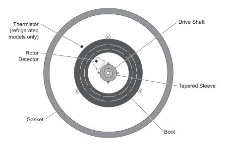
Figure 1-2. Interior View of the Rotor Chamber
