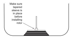
Figure 3-1. Tapered Sleeve Position
