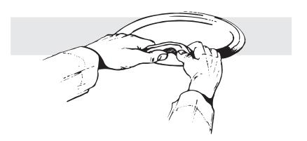
Figure 5-1. Replacing the Rotor Chamber Gasket
