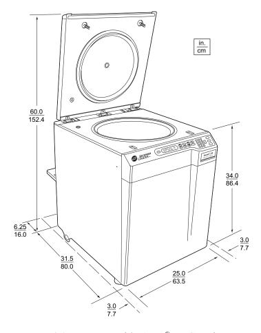
Figure 2-1. Dimensions of the Avanti® J-E Centrifuge
