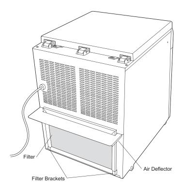
Figure 5-1. Air Filter Replacement
