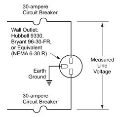
Figure 2-2. Single-Phase Power Connection
