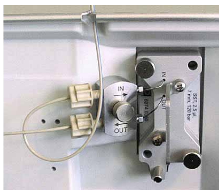
Fig. 39: Analytical flow cell with PEEK inlet capillary
