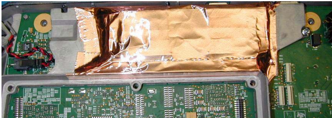
Figure 4.18 Copper Tape Installation - 3rd Strip
