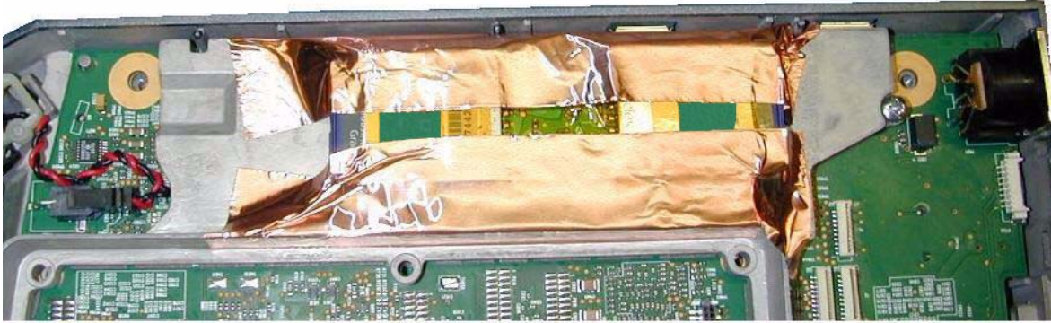
Figure 4.17 Copper Tape Installation - 2nd Strip
