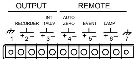
Figure 8 Input/Output Terminal
