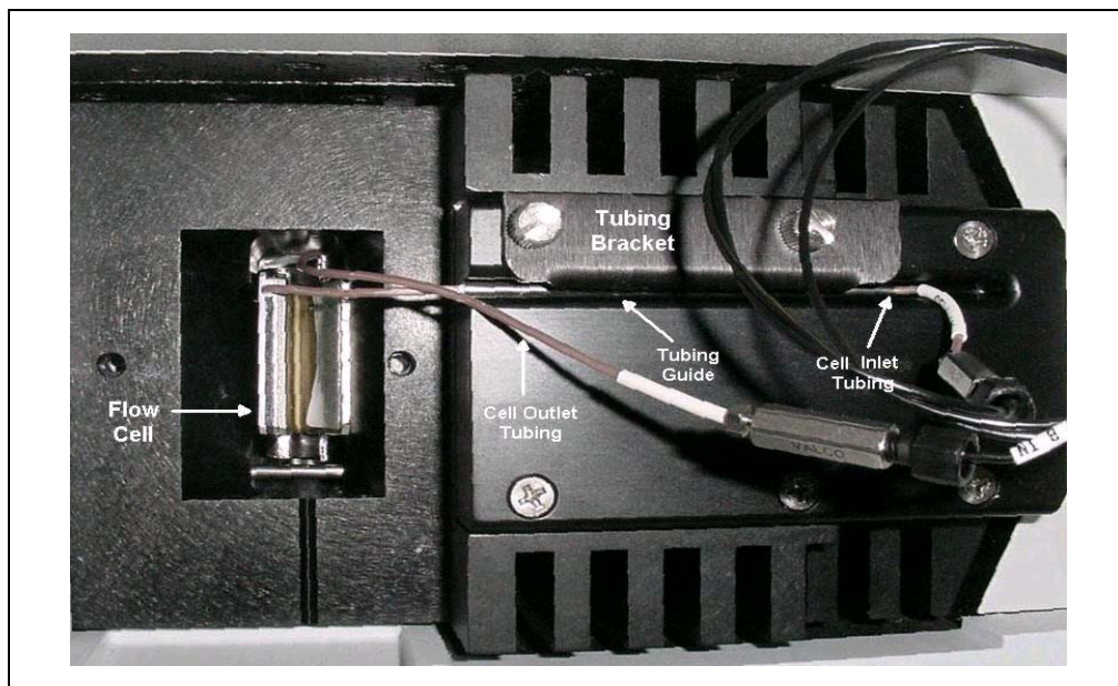
Figure 5-1. Removing the Flow Cell from the Optical Bench (Flow cell cover not shown)
