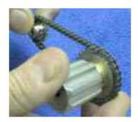
6. Install the chain and sprockets onto the needle valve stems as an assembly. Press the  $O_2$  knob/sprocket against the  $O_2$  minimum stop collar.
