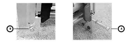
**Note** The flowmeter modules are held together at the top with a u-clip. To separate the modules, pivot the modules (front to back) 45 degree. The u-clip will disengage and allow the modules to separate.
