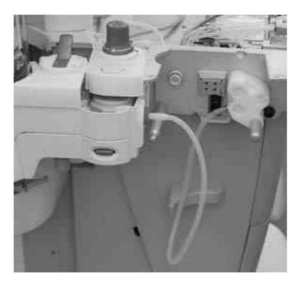
Test 7 Testing the bellows, the bellows pop-off valve, the bellows base manifold, and the Bag/Vent switch
