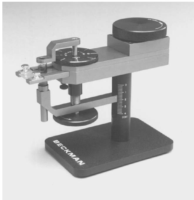
**347960** CentriTube Slicer Kit. Includes Adapter Plates, Blades, Storage Box, Hardware Kit, Spinkote™ Lubricant, and Instruction Manual.
