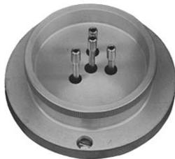
The Seal Assembly holds the lines through which fluids are introduced and withdrawn while the rotor is spinning at 2000 rpm. The assembly may be used with any of the Beckman Coulter zonal rotors in any Beckman Coulter preparative ultracentrifuge.
