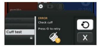
• A test error also briefly causes a yellow "LOW PRESSURE" warning tile to appear as well as the cuff status bar changing yellow. These warnings close after the Error view appears.
