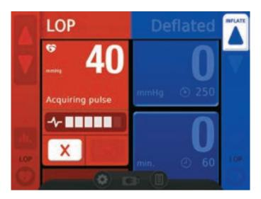
If the sensor or cuff was not properly installed, or an error occurs, the unit will display a warning window and alarm messages similar to the example below:
