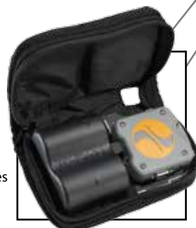
Amplifier pouch with a 32 channel EEG amplifier.
