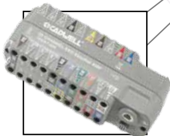
Amplifier pouch with a 32 channel EEG amplifier.
