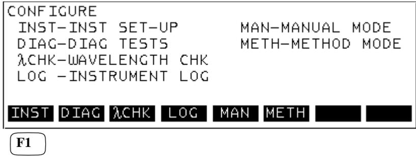
**2** Press F1 **INST** to move to the Instrument Setup Screen.
