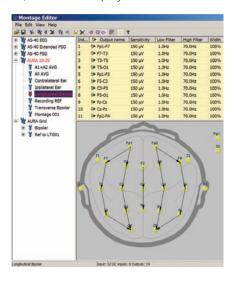
create bipolar output montages by Row or Column. User-defined average-reference montages, channel types, and trace colors can also be defined. The Montages used for a given study are also stored with the EEG data for retrieval during review or in the future when reviewing archived data.
