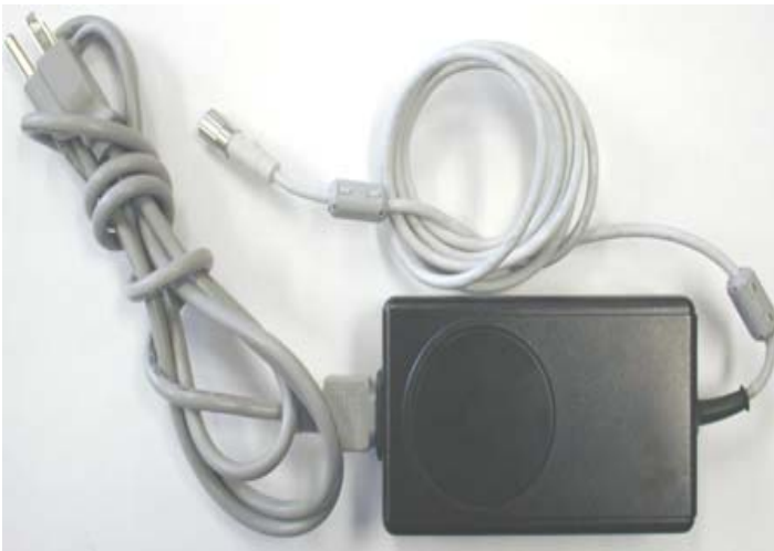
Figure 10. external medical grade ac/dc adapter
