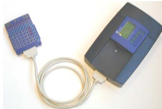
Figure 4. headbox to amplifier cable
