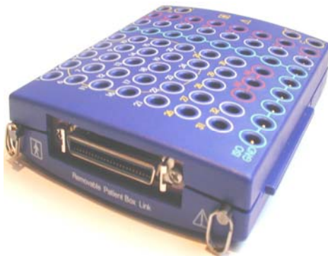
Figure 3. removable patient box (headbox) link port
