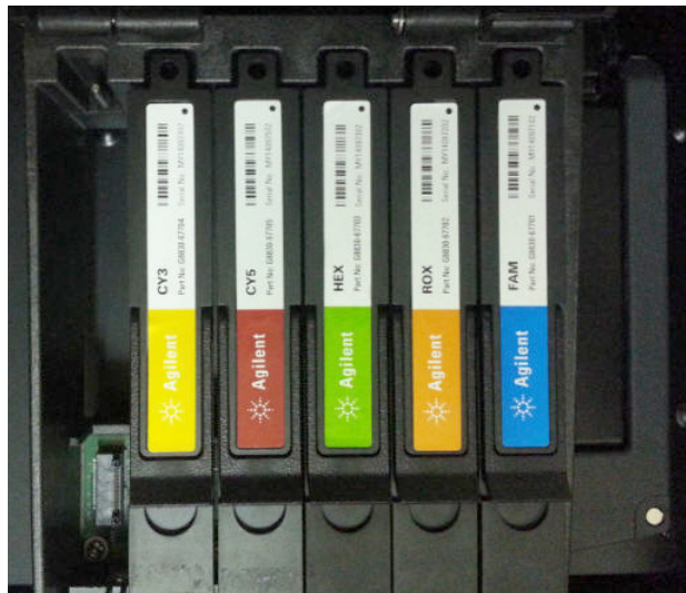
Figure 10 Installed optical modules
