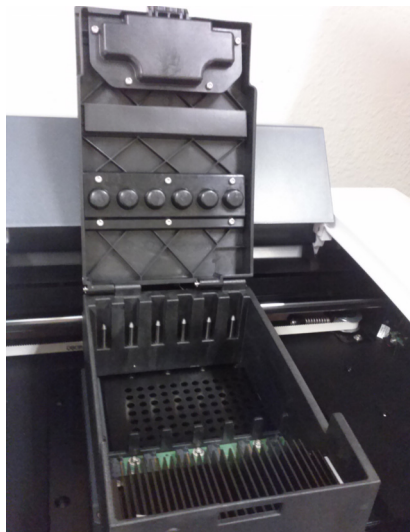
Figure 7 Slots for the optical modules
