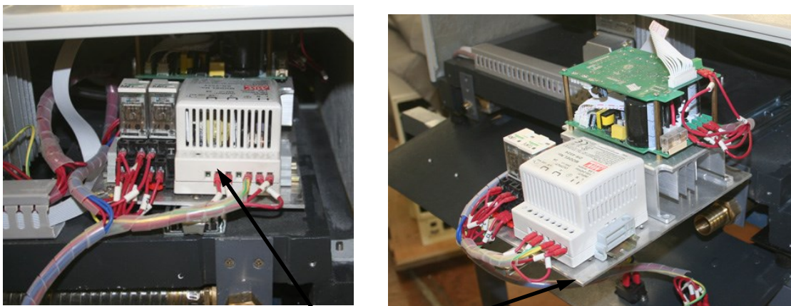
Easy access to electronics with sliding rail design
