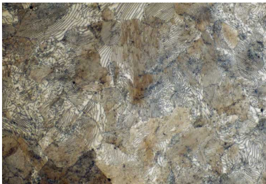
1095 Steel, Furnace-Cooled, etched with 2% nital, 400X B.F.
