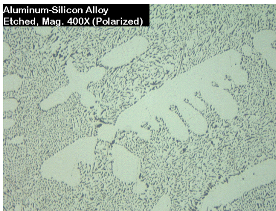
Aluminum - Silicon Alloy microstructure, Kallings etchant
