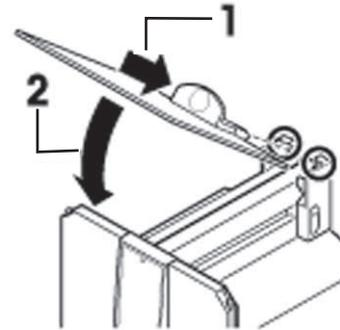
► The handles (A) must be turned toward the outside to allow installation of the side draft shield doors!
