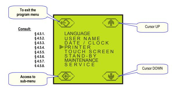
... Place the cursor ">" in front of the desired sub-menu using the "UP" and "DOWN" keys. Confirm the selection by pressing the sub-menu access key.
