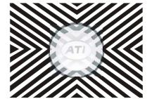
The result is also incorrect, if the indicator is grey or silver (over-exposure, i.e. excessive temperature).
