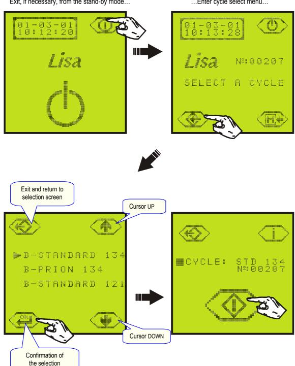
Position the cursor in front of the required cycle. Confirm your selection by pressing the "OK" key.
