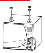
If the sterilizer is not used for more than 3 days, both water tanks must be completely drained in order to avoid alga growth or any other deposits.
