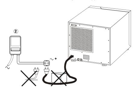
Plug in the mains cable to the back of the sterilizer.
