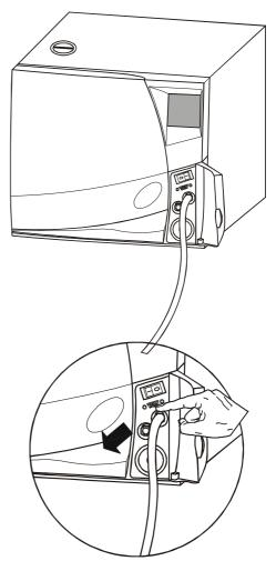
If the sterilizer is not used for more than 3 days, both water tanks must be completely drained in order to avoid alga growth or any other deposits.
