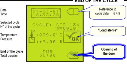
At the end of the cycle, the micro-processor analyses the temperature, pressure and duration of all the phases in order to confirm whether or not sterilization has occurred. After reading the comment, you can open the door by pressing the corresponding key.
