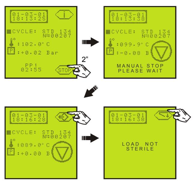
...This is followed by a phase of approximately 2 minutes, required to reinitialise the system and return the chamber to atmospheric pressure.
