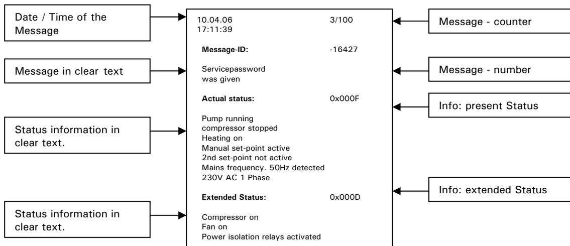
By turning the rotary knob / key (61) one can display the individual messages. Take note of the message counter for reference.
