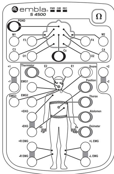
2. Make sure to connect other sensors to the bipolar channels as specified in the acquisition application.
