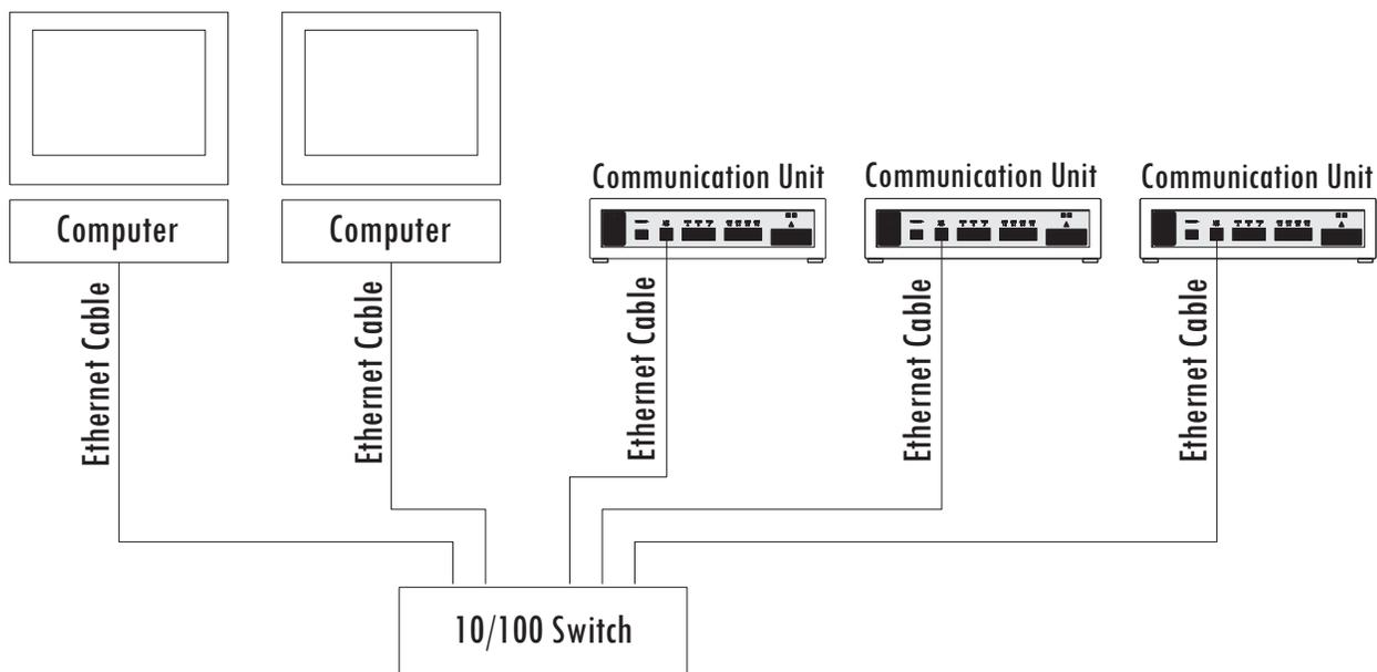
Schematic diagram of a typical Embla S4500 network
