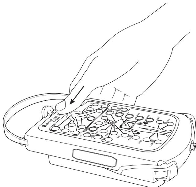
*Securing the Bedside Unit in the bracket*
