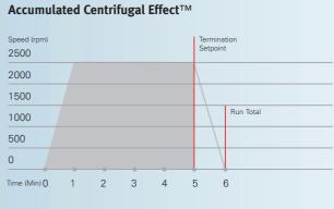
The ACE function ensures that all samples experience the same Total Centrifugal Effect (the area under the speed/time curve) by adding or subtracting time to a run.
