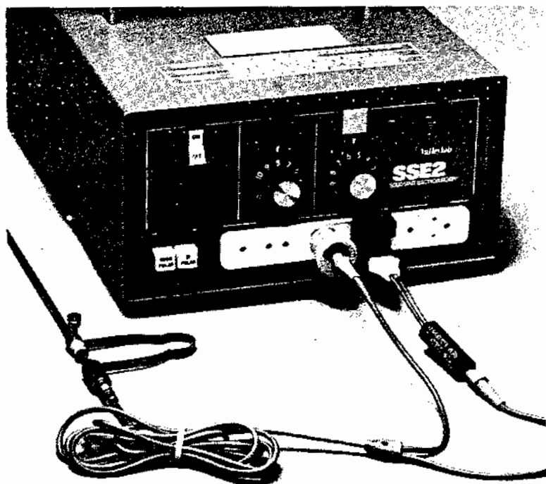
E0021 Adapter shown plugged into the REM patient return. This adapter allows the monopolar output to be used in a macrobipolar procedure with a REM equipped generator.
