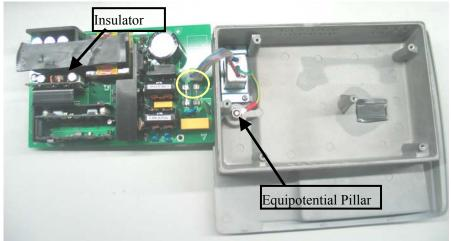
• Because the power supply board may be adhered to the insulator, be careful not to damage the parts, connector and cables when prizing it.
