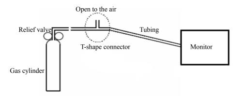
4. Open the relief valve and vent a certain standard gas or gas mixture and make sure that there is an excess gas flow through the T-shape connector to air. And wait for at least 30 seconds until the gas reading stable.
