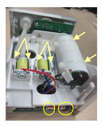
5. Unscrew the two M3×8 screws on the parameter board. Then pull off the parameter board rightward as shown below.
