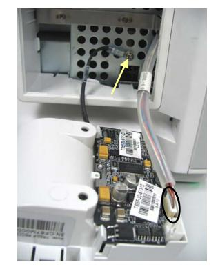
3. Unscrew the  $M3 \times 6$  screw and remove the cables marked in the picture.
