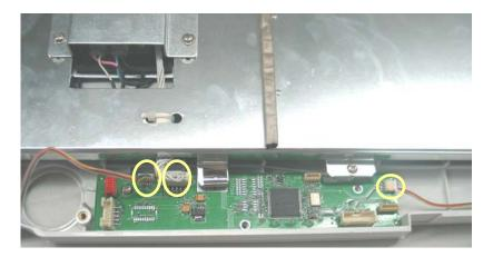
2. Remove the grounding spring and then unscrew the three PT3×8 screws and take out the button board.
