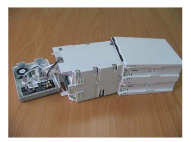
3. Hold the housing with both hands. Press the snap side with the thumb and move the other side with the index finger and the middle finger to separate the housing into two halves.
