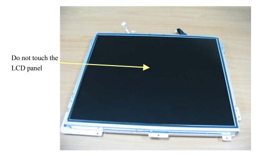
2. Unscrew the four M3  $\times$  6 screws and take out the LCD screen.
