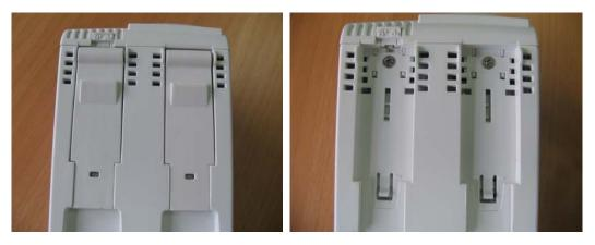
Take off the front cover of the CO<sub>2</sub> module by referring to the procedure as described in *5.6.1 Disassembling the ICG Module*. Then press the two clips about 1mm and take off the housing.
