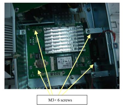
2. Remove the SSD hard disk and battery from assembly
