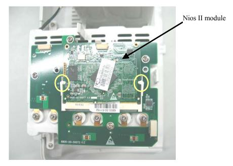
5. Unscrew the four M3 $\times$ 6 screws and take out the 3-slot module rack communication board. Unscrew the four M3 $\times$ 6 screws and take out the MPM Communication Board.
