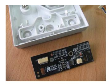
6. Unscrew the two screws on the front panel. Disconnect the tubing between the watertrap assembly and CO<sub>2</sub> parameter board. Disconnect the cable between the watertrap and CO<sub>2</sub> parameter board. Then take out the watertrap connector assembly.
