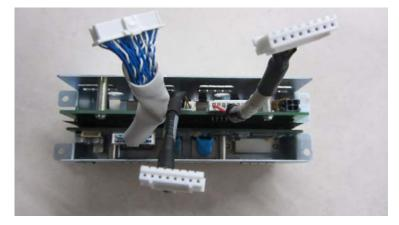
1. Unscrew the four  $M3 \times 6$  screws and remove the interface board assembly.
