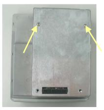
5. Unscrew the two M3×6 screws. pry out the board with a small flat-bladed screwdriver in the gap between the power supply board and the housing. Then turn the board over and unplug the cables from it.
