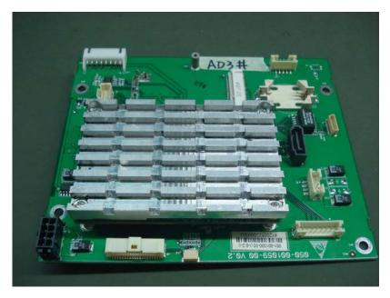
3. Unscrew the four pan head cross recessed screws and remove the cooling fin in the industrial control board.
