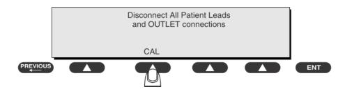
If the calibration fails, the previously stored readings will be used until a passing calibration has occurred. Also, the esc/stop key has no effect during calibration.
