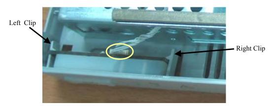
2. Release the clips with fingers. At the same time pinch the power switch & LED board, push it to the left and take it out along with the power switch.
