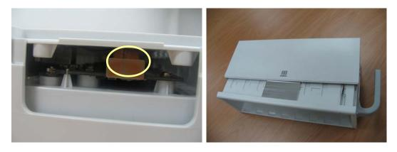
4. Unclench the two clips and take out the module rack interface board. Be sure not to damage the snap slot on the left side.
