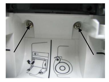
1. Open the recorder door and unscrew the two  $M3 \times 6$  screws.
