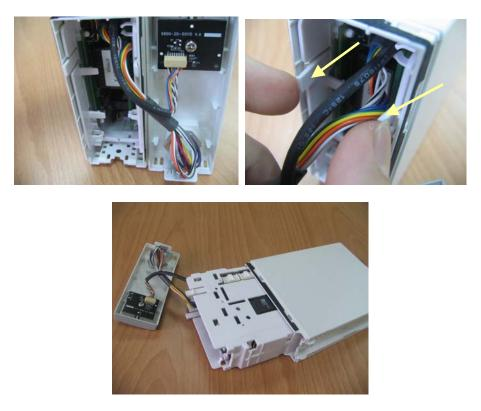
5. The side cover of the module without the housing is composed of two halves. Release the three snaps to separate the two halves.
