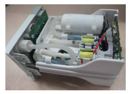
3. Disconnect the cable of the infrared communication board, and release the snap lock to remove the infrared communication board.
