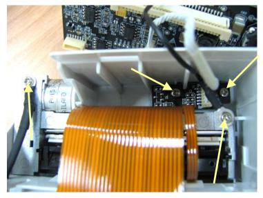
7. Remove the recorder mounting bracket by pulling out the recorder mounting bracket from the right side first.
