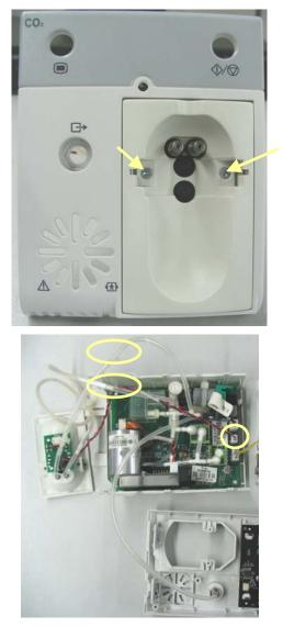
7. Disconnect the tubing between the CO<sub>2</sub> parameter board and the front panel. Then release the four clips and remove the CO<sub>2</sub> parameter board.
