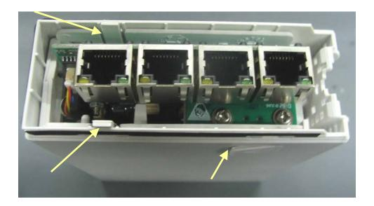
3. Release the three snaps to separate the two halves of the module side cover.
