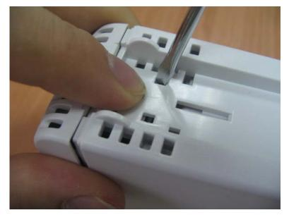
4. Press the two clips about 1mm and take off the housing.
