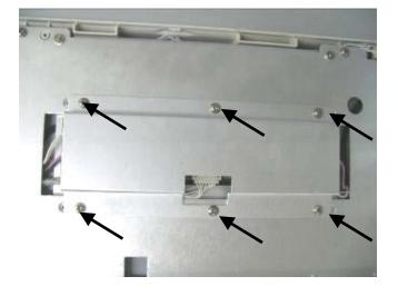
1. Unscrew the six  $M3 \times 6$  screws and remove the inverter shield.
