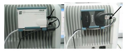
1. Disconnect the network cable and the power cord
