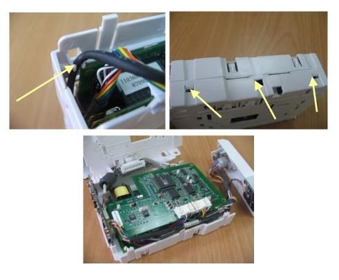
6. Take out the non-insulated power board and disconnect all the cables from it.
