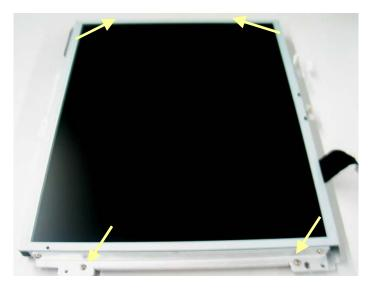
3. Unscrew the four M3 $\times$ 6 screws and separate the LCD screen from the two supporters.
