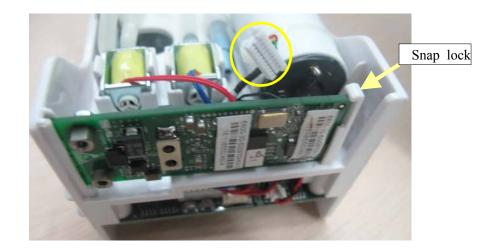
4. Disconnect the cables of the NIBP inflation pump and the relief valves from the parameter board. Snip off the cable ties to remove the pump. Release the snap locks to remove the valves.
