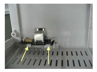
5. Remove the cable that connects the 8-slot communication board and the LED board, the LED indicator and the light tube.
