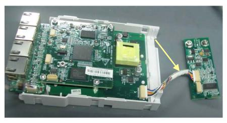
6. Unclench the four clips with a tweezer to remove the interface board.
