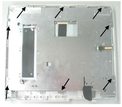
Unscrew the twelve  $M3 \times 6$  screws of T9 monitor and take the screen assembly out carefully. To prevent the screen from being contaminated by dust, do not touch the screen.
