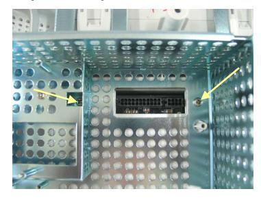
3. Lift the power supply assembly slightly to separate it from the two shafts on the rear cover and then remove the assembly.
