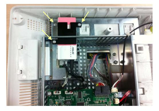
2. Unscrew the two  $M3 \times 6$  screws and then remove the wireless AP.
