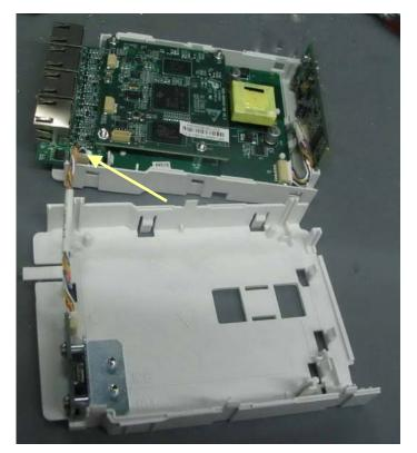
5. Take off the cable between the infrared communication board and the interface board to remove the infrared board.
