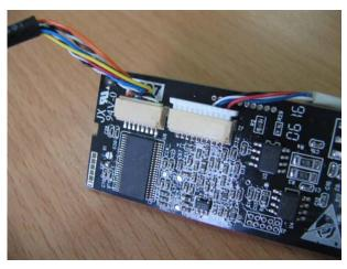
8. Disconnect all the cables on the ICG board and take off it with the front cover.
