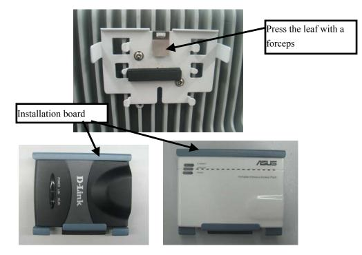
3. Unscrew the two  $M3 \times 8$  screws and take out the fix board.
