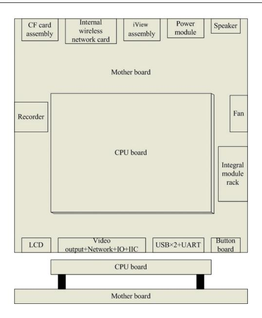
The CPU board is an essential CPU system containing the CPU, FLASH, memory, realtime clock, EEPROM, etc. It interfaces to the mother board only, which then provides interfaces to all other external devices.
