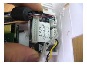
7. Take out the infrared communication board and disconnect all the cables from it.
