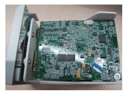
6. Unscrew the two  $M3 \times 4$  screws on the SpO<sub>2</sub> board to separate the SpO<sub>2</sub> board and the parameter board.
