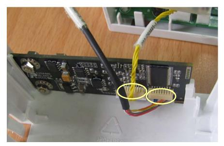
4. Take out the infrared communication board and disconnect all the cables from it.
