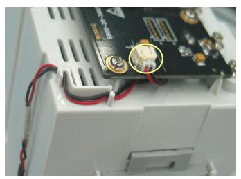
6. Unclench the clips and take out the Nios II module. Then unscrew the six M3×6 screws and remove the 8-slot module rack communication board.
