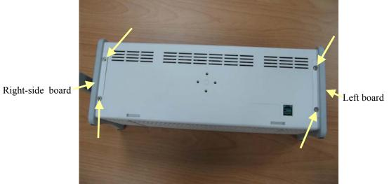
2. Pull off the left- and right-side boards. Be sure to place the rubber loop in position when
