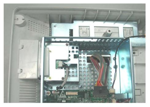
2. Unscrew the two  $M3 \times 6$  screws and take out the CF driving board.
