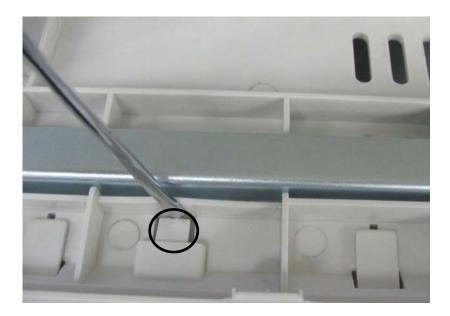
3. If the module rack still engages with the back cover, insert a small flat-bladed screwdriver into the position marked in the picture and pry it out about 1mm to release the hidden snap between the integral module rack and the back cover. Then pull out the module rack.
