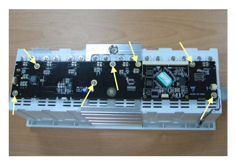
7. Use the sleeve to unscrew the hexagon nut and countersunk external toothed lock washer assembly which can be further separated into the washer, springlet and contact screw.
