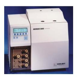
The oven has a front opening door for easy access to a maximum of three columns. Dynamic air flow eliminates temperature gradients across the oven. An overheat protection circuit prevents thermal runaways caused by spiking or surging line current.
