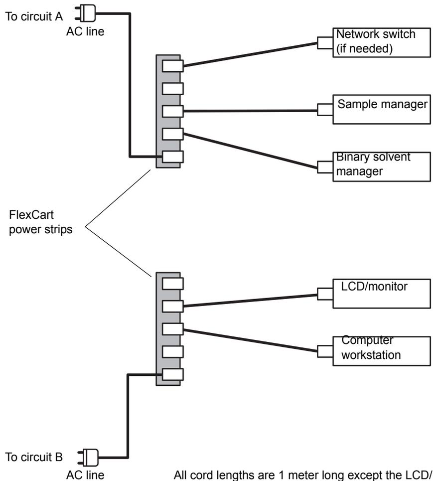
All cord lengths are 1 meter long except the LCD/monitor cord, which is 2 meters long.
