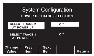
Press the **Change Value** softkey to scroll through the available parameters for each Trace selection.
