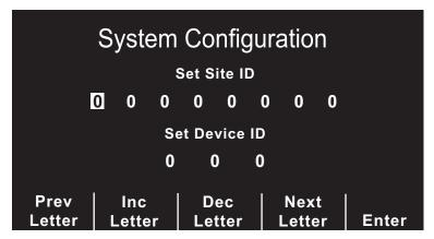
Pressing the **Prev Letter** softkey moves the highlight left to the previous entered digit. Pressing the **Inc Letter** or **Dec Letter** softkeys increments or decrements the selected digit. Pressing the **Next Letter** softkey moves the highlight right to the next digit to be entered. Pressing the **Enter** softkey selects the values that have been entered and returns to main configuration menu.
