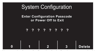
Users entering System Configuration for the first time must enter the default passcode (0000000) for System Configuration to continue.
