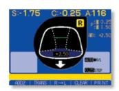
4 Move the lens table to align he glasses along the near-point section. The (+) target quickly follows your movement and the right and left arrows indicate if the lens needs to be centred. When reaching the maximum ADD, the (+) target will change.
