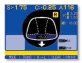
2 Align the lens so that the (+) target is centered.
