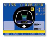
**3** As soon as the target is aligned, the lower section of the hourglass indicates the reading for distance Rx and automatically memorises it.
