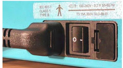
Prior to applying power to the instrument, make sure that the power cord is plugged firmly into the power entry module by pressing the cord connector into its receptacle.
