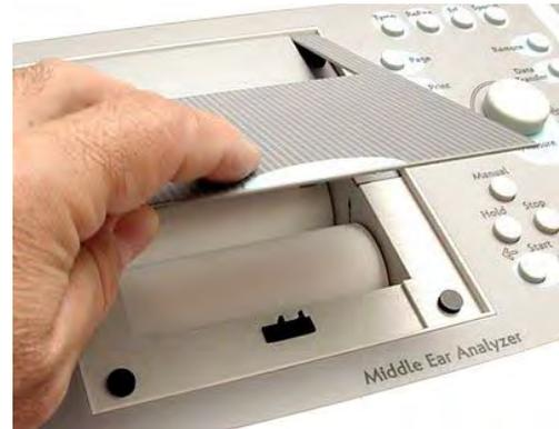
If it is necessary to replace a nearly exhausted roll of paper, rotate the release lever on the left side of the printer to its “back” position and gently pull the remaining paper out of the printer.
