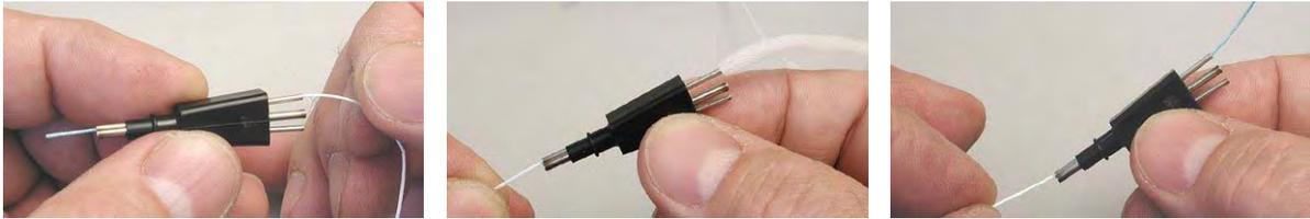
Reconnect the tygon tubing to the probe tubes. The center tube has the larger diameter.
