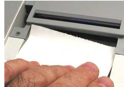
Orient the new paper roll as shown on the inside of the paper tray, rotate the release lever back to the “forward” position and feed the paper into the printer paper entrance until the printer motor and roller pulls the paper into the printer.
