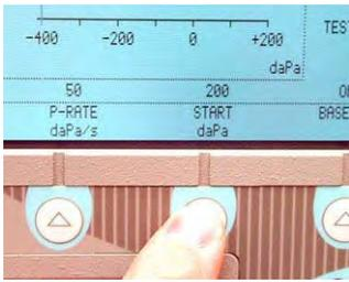
Pressing a parameter menu softkey causes a sub-menu of parameter settings to be displayed. Often sub-menus will contain MORE softkey selections that provide access to additional setting alternatives.
