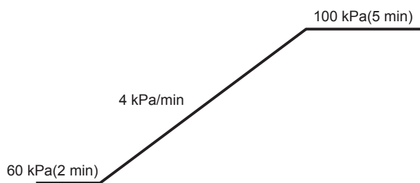
Fig. 12.2.9 Pressure program example
