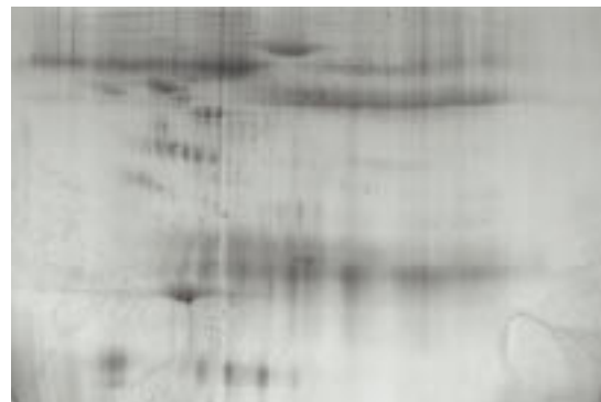
Protein stained with SYPRO® Ruby after 2D electrophoresis (473nm excitation laser with LPG filter)
