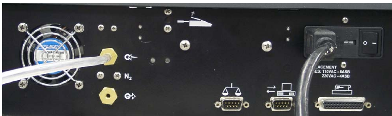
Dry Air Inlet with Tygon 2075 tubing connected
