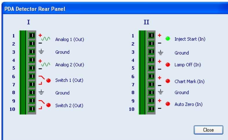
The following table describes the PDA detector I/O connections.
