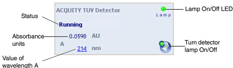
The TUV detector control panel displays absorbance units and wavelength values. You may edit these when the system is idle by clicking on the underlined value. You cannot edit detector parameters while the system is processing samples.
