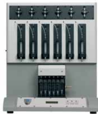
The AutoTrace 280 instrument provides automated solid-phase extraction with a choice of cartridge or disk formatting.
