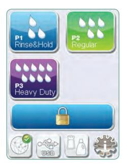
A high-resolution, 65K color touch screen offers a vivid display of messages, current cycle information and customizable colors all with extraordinary clarity. Fully adjustable contrast levels let you optimize the screen to the lighting in your steri-center, and it's 2.5-inch by 3-inch dimensions allow easy viewing of cycle information.
