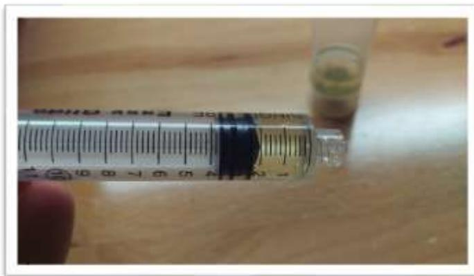
19. Place syringe on syringe filter at sample port by gently twisting it on about a quarter turn. Press forward arrow on screen.
