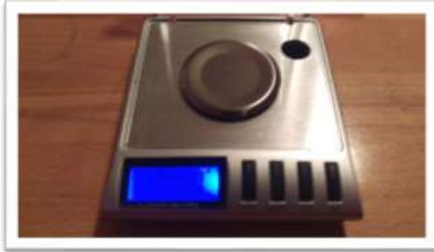
2. Press and hold ON button for about 3 seconds until CAL is displayed on screen. Press ON button once more.
