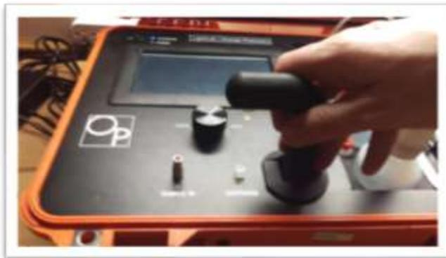
Press Start button to turn on pump. LightLab will flush solvent for 90 seconds.
