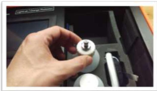
2. Detach solvent fluid line and remove solvent cap. Remove solvent bottle and replace storage cap. Remaining solvent can be added to waste bottle.
