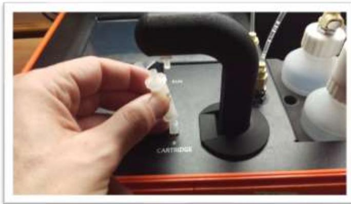
3. Remove caps on new column and place into column holder.
