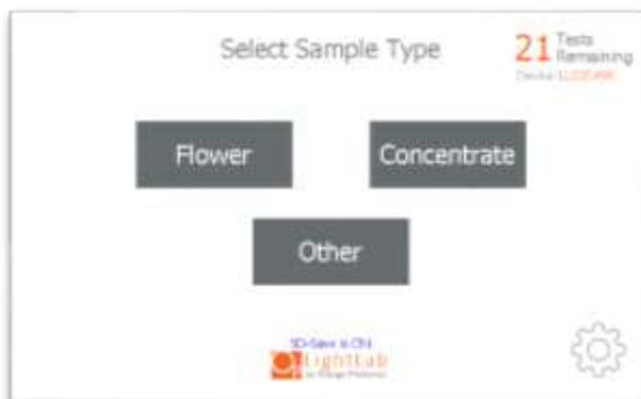
2. Select the type of sample to be measured from the new list that appears (Custom for this section). NOTE: if tests remaining is zero, you will be prompted to replace the column, see Section 11
