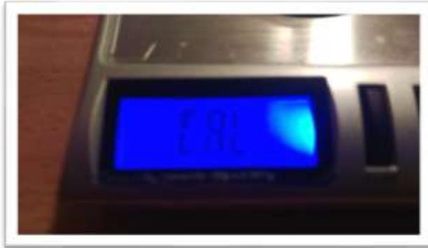
3. After a few seconds, the display will flash 10.000. Add the first calibration weight to the scale.
