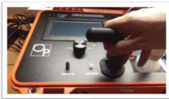
2. Remove sample fluid lines from solvent and waste bottle. Replace with flushing lines. The flushing lines have opposing male and female ends. The solvent bottle should be connected to the OUT on the instrument and the waste should be connected to the IN on the instrument. Press forward arrow on screen.
