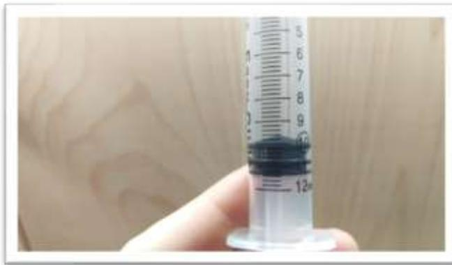
13. Add contents of syringe to vial and place cap firmly on vial. Press forward arrow on LightLab screen.
