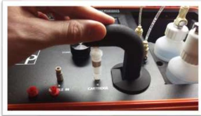
5. LightLab will flush new column for 90 seconds, and will be ready for a new sample once complete.
