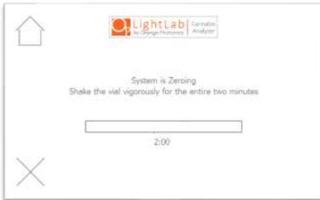
16. Once Zero is complete, add syringe filter onto sample port. Note some samples may require larger filters. Press forward arrow on screen.
