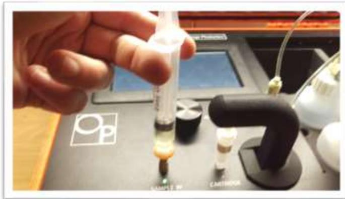
21. Set valve to Run. Press forward arrow on screen.
