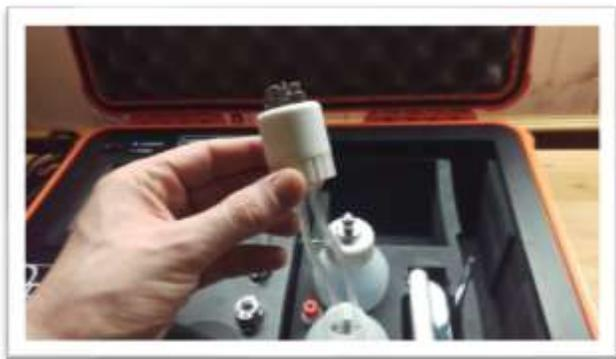
3. Add new solvent and waste bottles and reconnect fluid lines.
