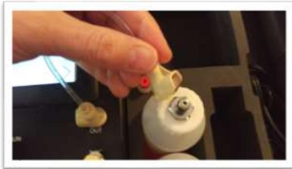
4. Connect waste line to sample input flush port on the side of the instrument. Press forward arrow on screen.
