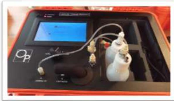
7. Press Start button to begin flush. The LightLab solvent should come out of the Sample In port and into the waste bottle, forcing any debris in the fluid lines with it.
