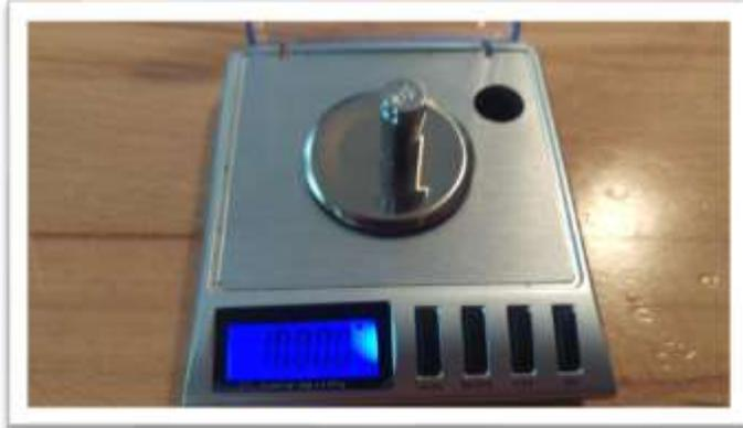
7. Place a vial cap on the scale and press "tare". Ensure scale now reads zero with cap resting on it. Press forward arrow on the LightLab screen.
