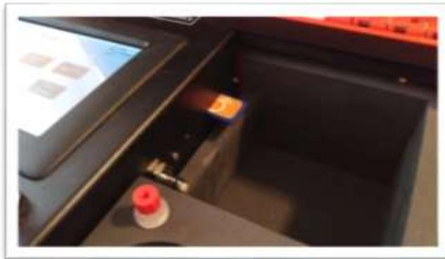
When the SD card is inserted, test results are automatically saved to the SD card in a comma separated value (Excel compatible) format. If the SD card is removed during testing, it is still possible to access test results by using the Export Data function. The Export Data function also allows export of diagnostic data that can be used by Orange Photonics Support to help troubleshoot an instrument. To export data, follow these instructions:
