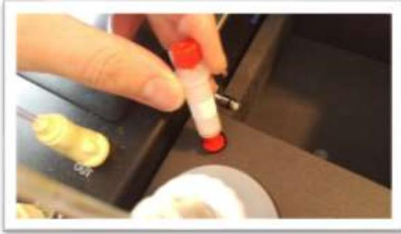
4. Remove fluid lines and place in cap baton. Placing them in partway and tapping the baton on the table allows them to slide to the bottom of the baton.
