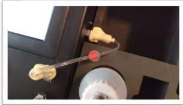
5. Connect Luer end of sample flush line to Sample In port. Press forward on screen.
