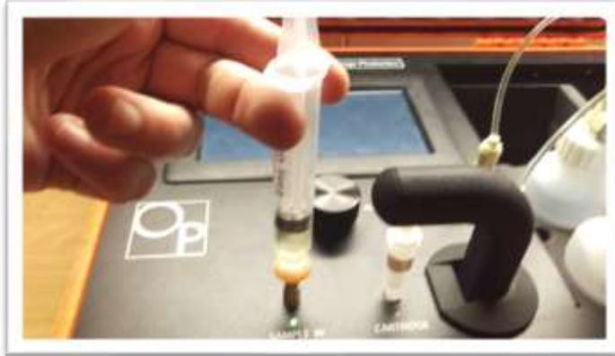
22. Set valve to Run. Press forward arrow on screen.
