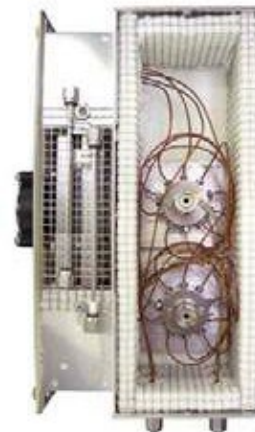
Dual TO-14 Concentrator (four traps, two valves)
